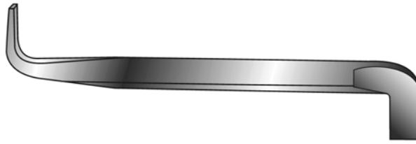
Fig. 2.36, Double-ended offset screwdriver.
