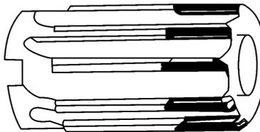
*Fig. 3.15, A carbide tipped shell reamer.*
