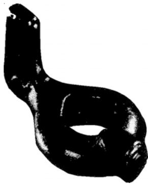
Fig. 6.25, Bent-tail dog with safety set screw.
