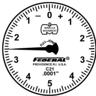
Fig. 2.68, Dial indicator test set.
