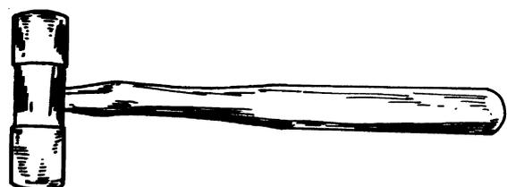
Fig. 2.21 (b), Plastic faced soft hammer.
