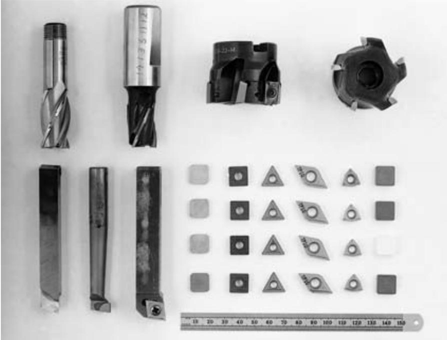
Fig. 1.12 Examples of turning and milling solid, brazed and insert tools
