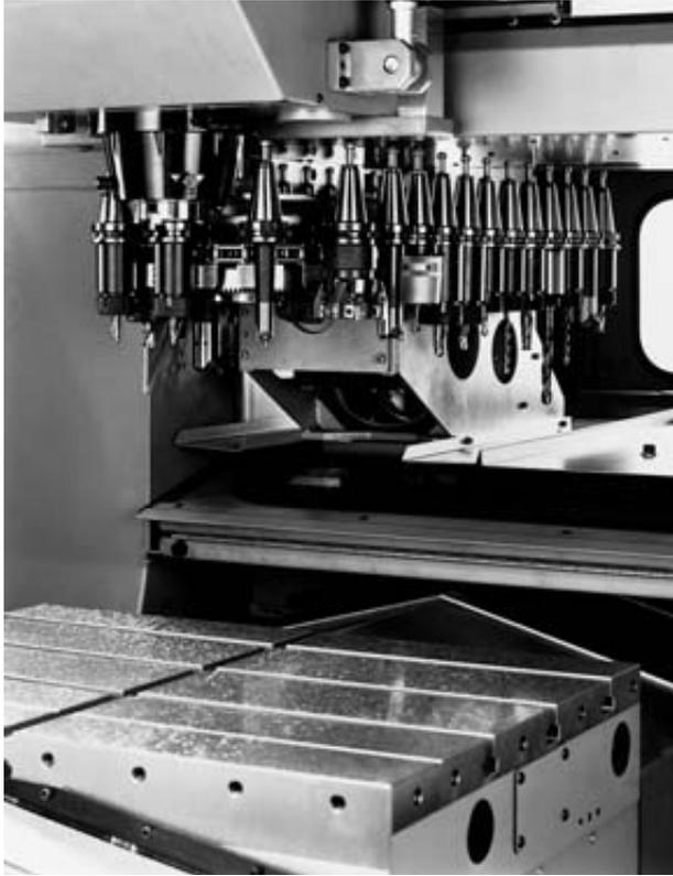
**Fig. 1.15** A milling machine tooling magazine
