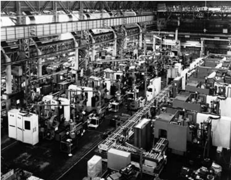
Fig. 1.17 Transfer line layout of an automotive manufacturing plant (after Hitomi, 1979), with a detail of a transmission case machining line
