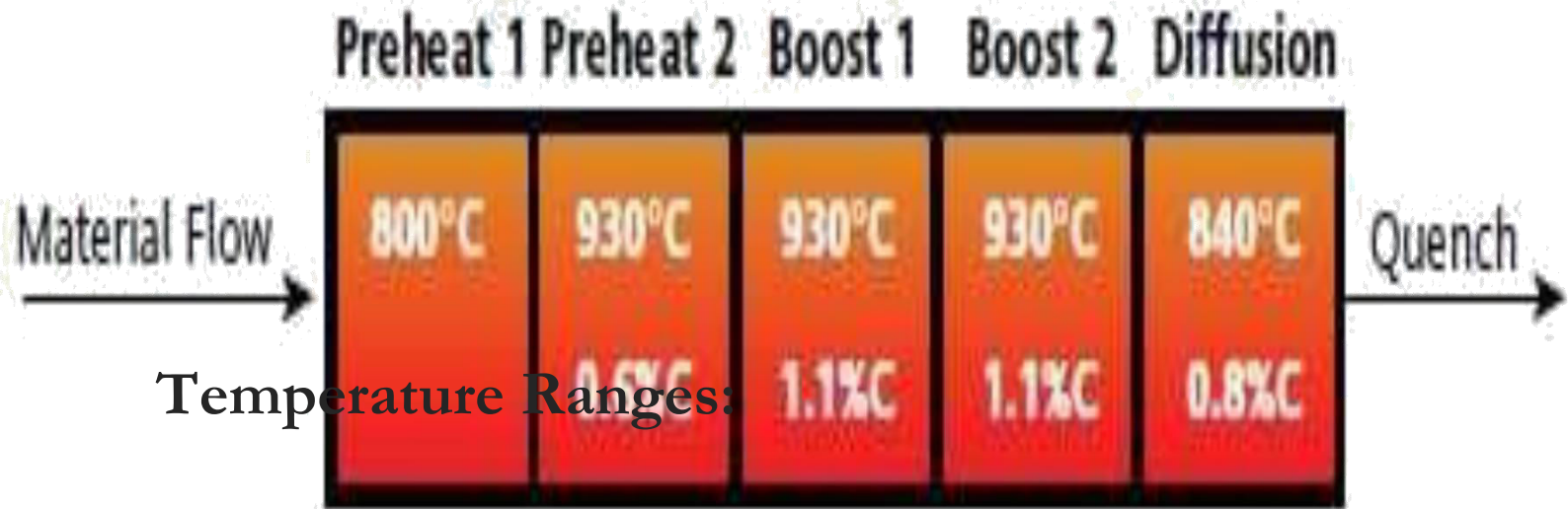
Fig.4.5 Heat flow in gas carburizing
