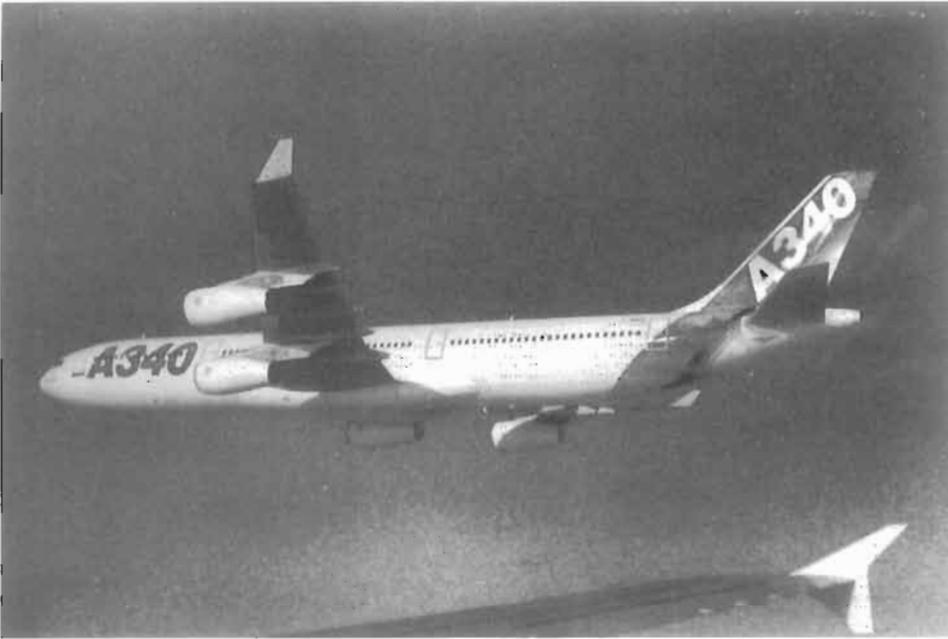
**Fig. 8.40** A view of the Airbus A340 showing the winglets attached to the wing-tips. These devices are used in order to reduce induced drag. See Fig. 8.37, page 523. In the foreground is the wing of the Airbus A320-200 fitted with another wing-tip device known as a wing-tip fence. (*The photograph was provided by Gert Wunderlich.*)
