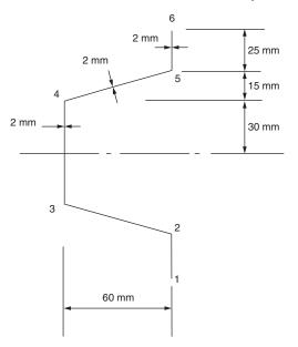
**P.17.12** A thin-walled closed section beam of constant wall thickness t has the cross-section shown in Fig. P.17.12.
