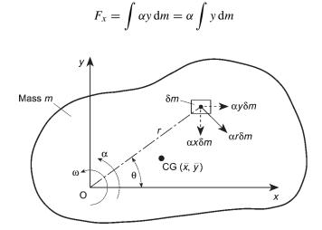
Fig. 14.2 Inertia forces on a rigid mass subjected to an angular acceleration.
