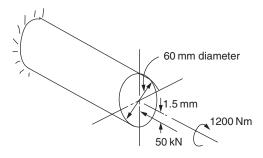
Fig. 1.10 Cantilever beam of Example 1.2.
