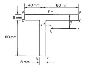
Fig. 16.13 Cross-section of beam in Example 16.4.
