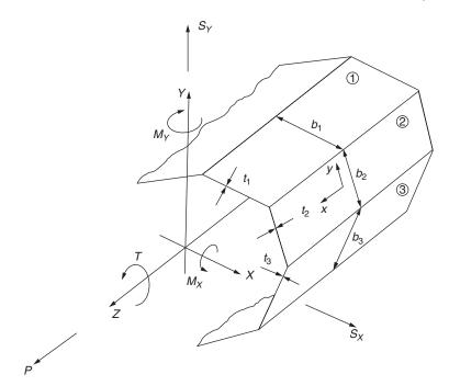
Fig. 25.9 Composite thin-walled section.
