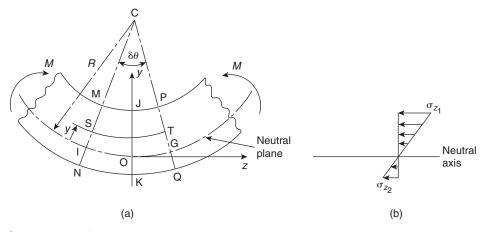
Fig. 16.5 Length of beam subjected to a pure bending moment.
