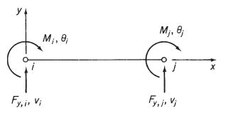
Fig. 6.6 Forces and moments on a beam element.
