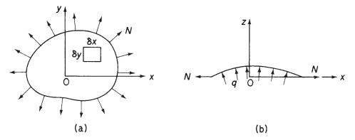
Fig. 3.7 Membrane analogy: in-plane and transverse loading.
