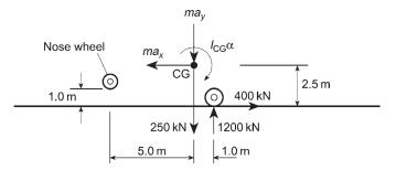
Fig. 14.5 Geometry of the aircraft of Example 14.2.
