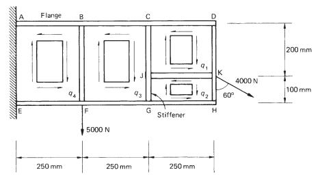
Fig. 24.1 Cantilever beam of Example 24.1.
