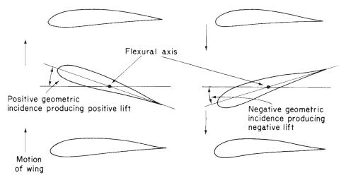
Fig. 28.7 Coupling of bending and torsional oscillations and destabilizing effect of geometric incidence.
