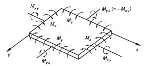
Fig. 7.4 Plate subjected to bending and twisting.
