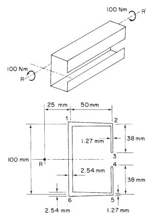
2.54 mm at their junctions with the web. The web has a constant thickness of 2.54 mm. The shear modulus G is  $26700 \text{ N/mm}^2$  throughout.
