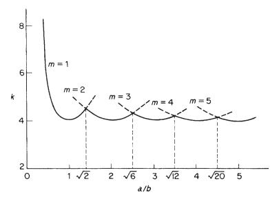
Fig. 9.2 Buckling coefficient k for simply supported plates.
