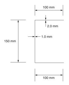
Fig. 25.10 Beam section of Example 25.4.
