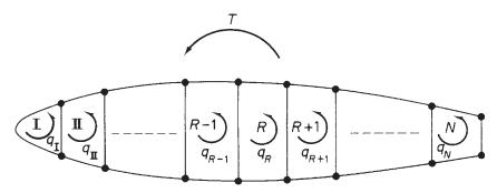
Fig. 23.4 Multicell wing section subjected to torsion.
