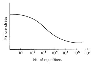
Fig. 13.2 Typical form of S–N diagram.
