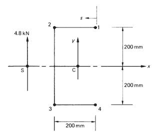
Fig. 20.7 Idealized channel section of Example 20.3.
