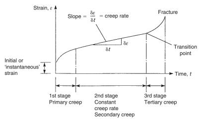
Fig. 11.18 Typical creep curve.
