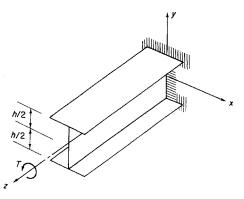
Fig. 27.4 Torsion of I-section beam fully built-in at one end.
