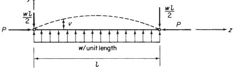
Fig. 8.11 Bending of a uniformly loaded beam-column.
