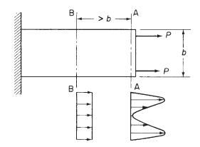
Fig. 2.4 Stress distributions illustrating St. Venant's principle.
