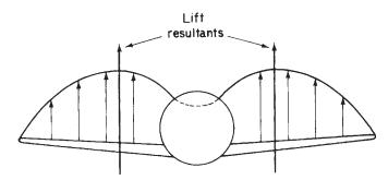
Fig. 12.3 Typical lift distribution for a wing/fuselage combination.
