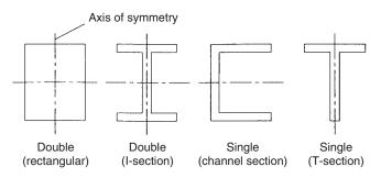
Fig. 16.2 Symmetrical section beams.
