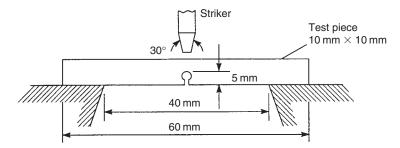
Fig. 11.8 Charpy impact test.
