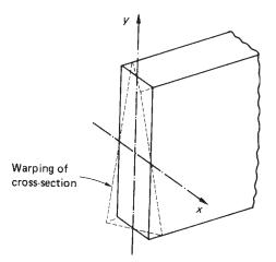
Fig. 3.10 Warping of a thin rectangular strip.
