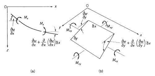
Fig. 7.14 (a) Strain energy of element due to bending; (b) strain energy due to twisting.
