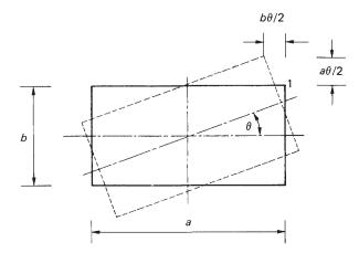
Fig. 18.8 Twisting of a rectangular section beam.
