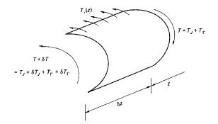
Fig. 27.17 Beam carrying a distributed torque loading.
