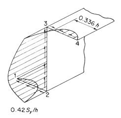
Fig. 17.7 Shear flow distribution in Z-section of Example 17.1.
