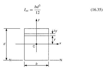
Fig. 16.27 Second moments of area of a rectangular section.
