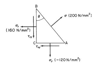
Now substituting the values  $\sigma_x = 160 \text{ N/mm}^2$ ,  $\sigma_y = -120 \text{ N/mm}^2$  and  $\sigma = \sigma_1 = 200 \text{ N/mm}^2$  we have
