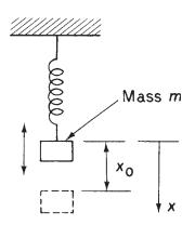
Fig. 10.1 Oscillation of a mass/spring system.
