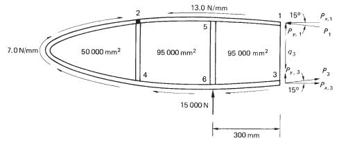
Fig. 24.13 Equilibrium of the rib forward of stiffener 31.
