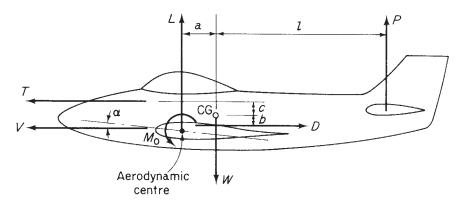
Fig. 14.6 Aircraft loads in level flight.
