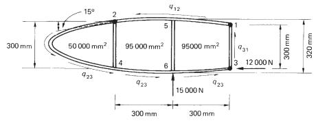
Fig. 24.9 Wing rib of Example 24.2.
