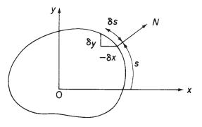
Fig. 3.2 Formation of the direction cosines *I* and *m* of the normal to the surface of the bar.
