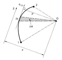
Fig. 20.10 Moment produced by a constant shear flow.
