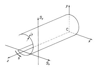
Fig. 17.5 Shear loading of open section beam.
