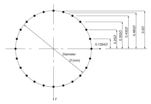
Fig. A.8 Idealized fuselage cross-section.
