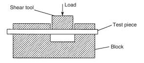
Fig. 11.5 Shear test.
