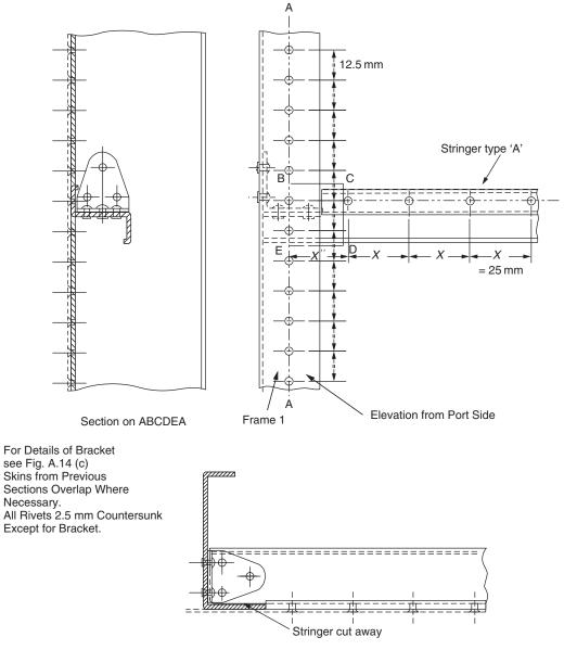
Fig. A.14(a) Detail, Frame 1.
