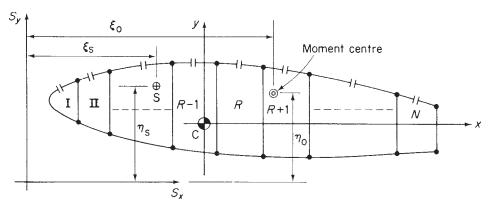
Fig. 23.8 N-cell wing section subjected to shear loads.
