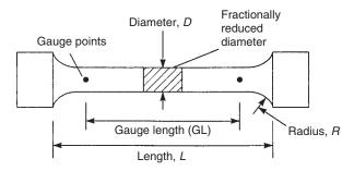
Fig. 11.2 Standard cylindrical test piece.
