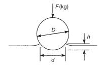
Fig. 11.6 Brinell hardness test.
