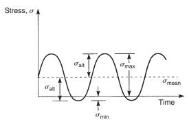
Fig. 11.20 Alternating stress in fatigue loading.
