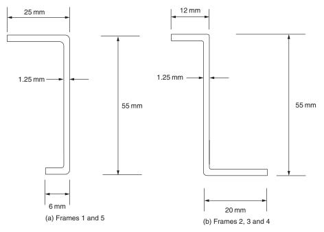
Fig. A.12 Fuselage frame sections.
