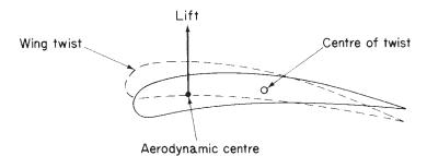
Fig. 28.1 Increase of wing incidence due to wing twist.
