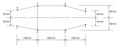
**P.20.3** Figure P.20.3 shows the cross-section of a single cell, thin-walled beam with a horizontal axis of symmetry. The direct stresses are carried by the booms  $B_1$  to  $B_4$ , while the walls are effective only in carrying shear stresses. Assuming that the basic theory of bending is applicable, calculate the position of the shear centre S. The shear modulus *G* is the same for all walls.
