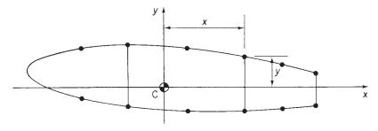
Fig. 23.2 Idealized section of a multicell wing.
