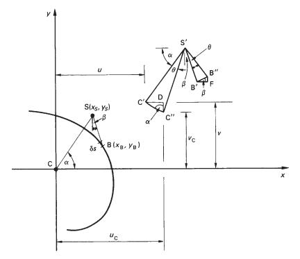
Fig. 8.16 Flexural-torsional buckling of a thin-walled column.
