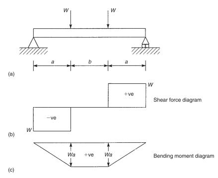
Fig. 11.3 Bending test on a beam, 'two-point' load.
