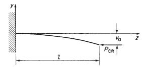
Fig. 8.15 Buckling load for a built-in column by the energy method.
