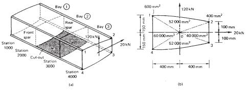
Fig. 23.21 Wing box of Example 23.7.
