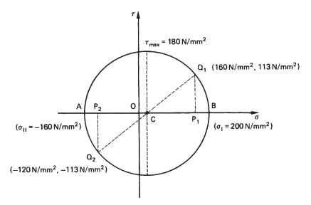
Fig. 1.14 Solution of Example 1.3 using Mohr's circle of stress.
