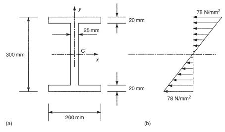
Fig. 16.6 Direct stress distribution in beam of Example 16.1.
