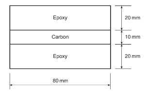
Fig. 25.4 Cross-section of the bar of Example 25.1.
