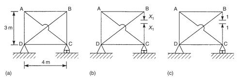
Fig. 5.22 Self-straining due to a temperature change.
