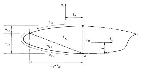
Fig. 23.1 Three-boom wing section.
