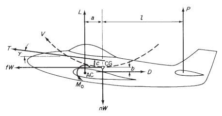
Fig. 14.7 Aircraft loads in a pull-out from a dive.
