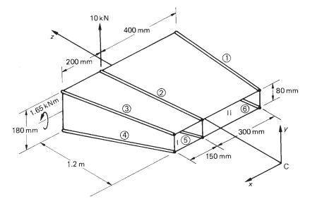
Fig. 23.12 Tapered beam of Example 23.4.
