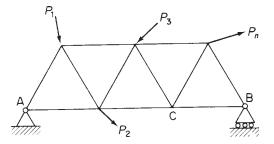
Fig. 5.3 Determination of the deflection of a point on a framework by the method of complementary energy.
