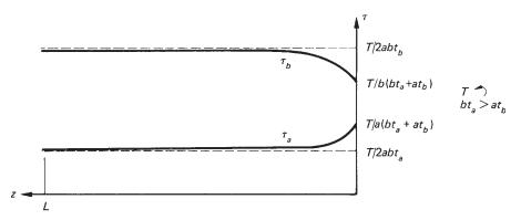
Fig. 26.9 Shear stress distributions along the beam of Fig. 11.5.
