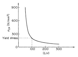
Fig. 8.6 Critical stress-slenderness ratio for a column.
