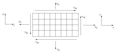
Fig. 25.6 Reference axes for a specially orthotropic ply.
