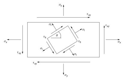
Fig. 25.8 Stresses in a generally orthotropic ply.
