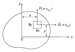
Fig. 3.3 Derivation of torque on cross-section of bar.
