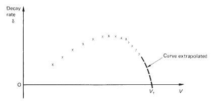
Fig. 28.11 Experimental determination of flutter speed.
