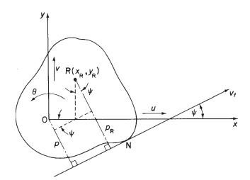
Fig. 17.4 Establishment of displacement relationships and position of centre of twist of beam (open or closed).
