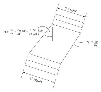
Fig. 26.29 Compatibility condition for the panel of Example 26.5.
