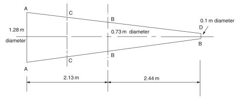
Fig. A.6 Rear fuselage sections.
