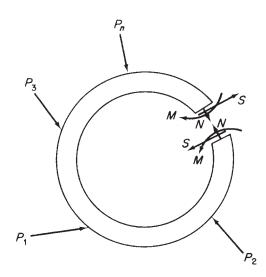
Fig. 5.13 Internal force system in a two-dimensional ring.
