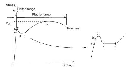
Fig. 11.9 Stress-strain curve for mild steel.
