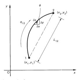
Fig. 20.9 Curved web with constant shear flow.
