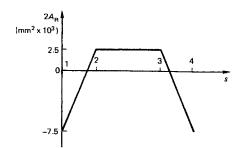
Fig. 27.21 Distribution of area 2A<sub>R</sub> in the column of Example 27.2.
