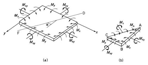
Fig. 7.5 (a) Plate subjected to bending and twisting; (b) tangential and normal moments on an arbitrary plane.
