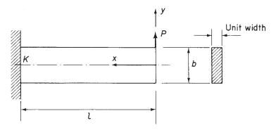
Fig. 2.6 Bending of an end-loaded cantilever.
