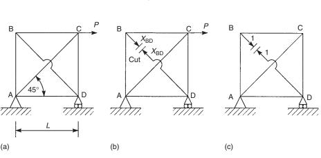
Fig. 5.20 Analysis of a statically indeterminate truss.
