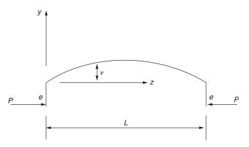
Fig. 8.10 Eccentrically loaded column of Example 8.2
