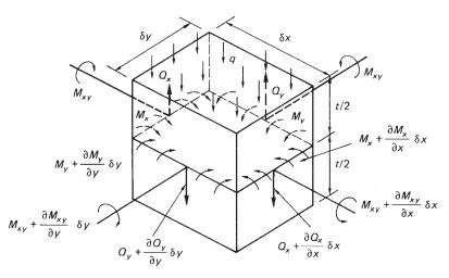
Fig. 7.9 Plate element subjected to bending, twisting and transverse loads.
