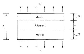
Fig. 25.2 Determination of Et.
