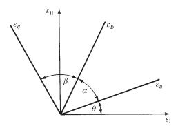
Fig. 1.18 Strain gauge rosette.
