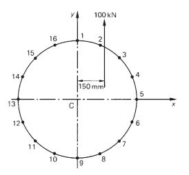
Fig. 22.2 Idealized fuselage section of Example 22.2.
