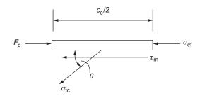
Fig. 9.18 Determination of flange stress.
