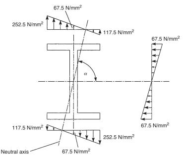
Fig. 16.7 Direct stress distribution in beam of Example 16.3.
