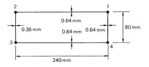
**P.20.5** A uniform beam with the cross-section shown in Fig. P.20.5(a) is supported and loaded as shown in Fig. P.20.5(b). If the direct and shear stresses are given by the basic theory of bending, the direct stresses being carried by the booms and the shear stresses by the walls, calculate the vertical deflection at the ends of the beam when the loads act through the shear centres of the end cross-sections, allowing for the effect of shear strains.
