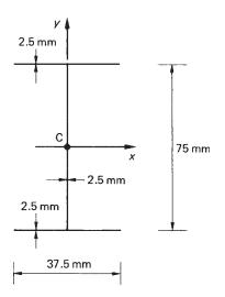
Fig. 8.17 Column section of Example 8.3.
