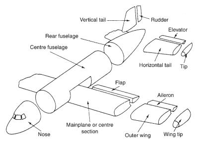
Fig. 12.8 Typical sub-assembly breakdown.
