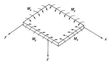
Fig. 7.1 Plate subjected to pure bending.
