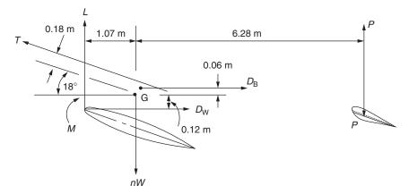
Fig. A.4 Balancing out calculations.
