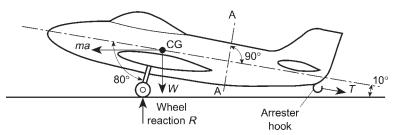
Fig. 14.3 Forces on the aircraft of Example 14.1.
