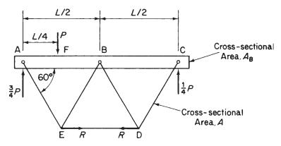
Fig. 5.12 Analysis of a trussed beam by the method of complementary energy.
