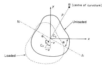
Fig. 16.15 Determination of beam deflection due to bending.
