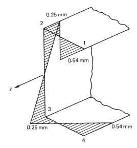
Fig. 18.13 Warping distribution in channel section of Example 18.3.
