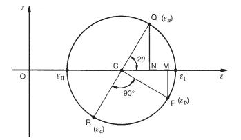
Fig. 1.19 Experimental values of principal strain using Mohr's circle.
