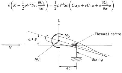
Fig. 28.2 Determination of wing divergence speed (two-dimensional case).
