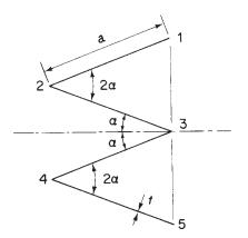
**P.17.3** Determine the position of the shear centre S for the thin-walled, open cross-section shown in Fig. P.17.3. The thickness t is constant.
