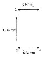
Fig. 20.8 Shear flow in channel section of Example 20.3.
