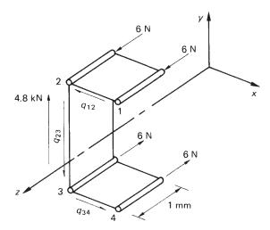
Fig. 20.13 Alternative solution to Example 20.3.
