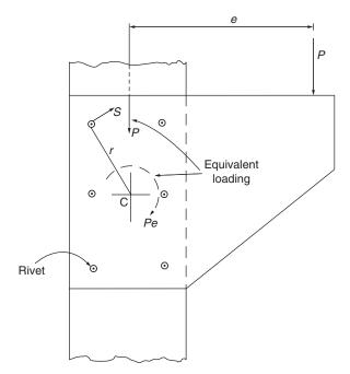
Fig. 12.14 Eccentrically loaded joint.
