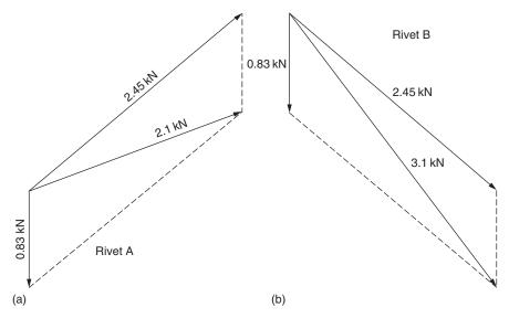
Fig. 12.16 Force diagrams for rivets of Example 12.2.
