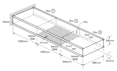
Fig. 23.16 Three-bay wing structure with cut-out of Example 23.6.
