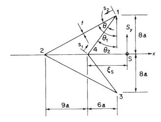
Fig. 17.13 Closed section beam of Example 17.3.
