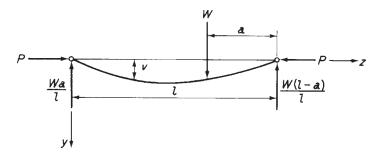
Fig. 8.12 Beam-column supporting a point load.
