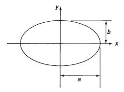
Fig. 3.6 Torsion of a bar of elliptical cross-section.
