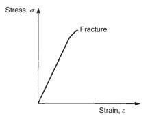
Fig. 11.15 Stress-strain curve for a brittle material.
