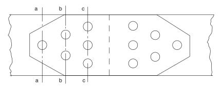
Fig. 12.13 A group-riveted joint.
