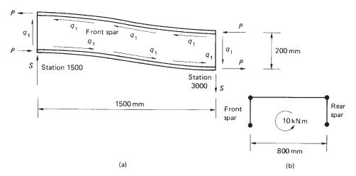
Fig. 23.17 Differential bending of front spar.
