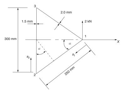
Fig. 25.12 Beam section of Example 25.6.
