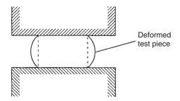
Fig. 11.12 'Barrelling' of a mild steel test piece in compression.
