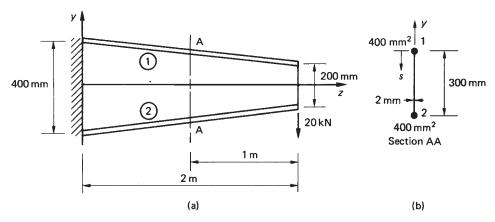
Fig. 21.2 Tapered beam of Example 21.1.
