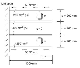
Fig. 26.22 Shear flows acting on top cover of idealized beam section of Example 26.4.
