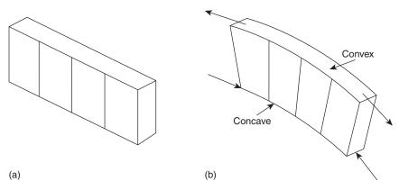
Fig. 16.1 Bending of a rubber eraser.
