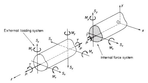
Fig. 16.10 Internal force system.
