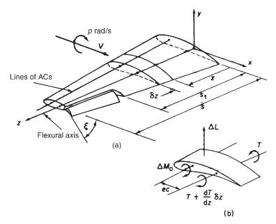
Fig. 28.6 Aileron effectiveness and reversal speed (finite wing).
