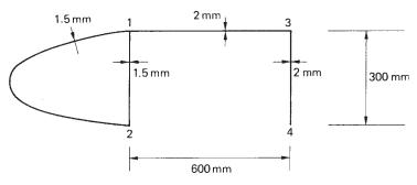
Fig. 19.4 Wing section of Example 19.2.
