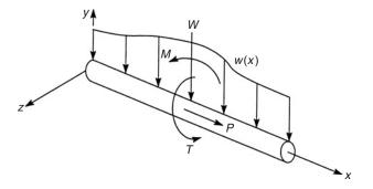
Fig. 4.7 Virtual work due to externally applied loads.
