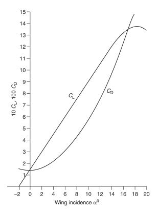
Fig. A.3 Wing characteristics.
