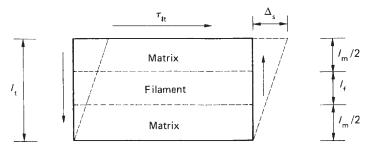
Fig. 25.3 Determination of G<sub>lt</sub>.
