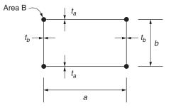
**P.26.7** In the panel shown in Fig. P.26.7 the area,  $A_s$ , of the central stringer is to be designed so that the stress in it is 80% of the constant stress,  $\sigma_e$ , in the edge members, each of area *B*.
