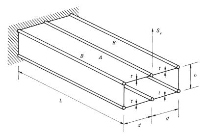
Fig. 26.11 Six-boom beam subjected to a shear load.
