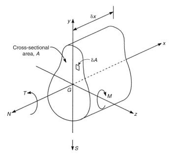
Fig. 4.5 Virtual work due to internal force system.
