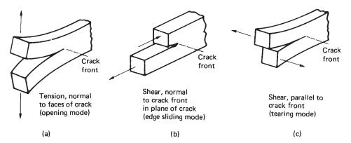
Fig. 15.4 Basic modes of crack growth.
