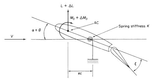
Fig. 28.5 Aileron effectiveness and reversal speed (two-dimensional case).
