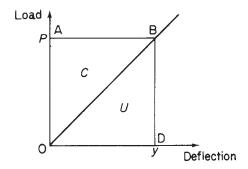
Fig. 5.2 Load-deflection curve for a linearly elastic member.
