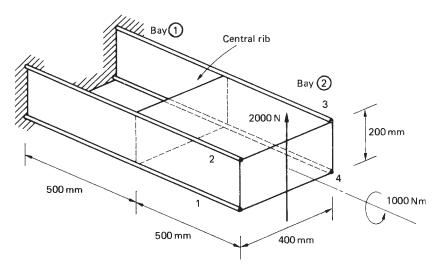
the skin panel in the upper surface of the inboard bay is removed, calculate the shear flows in the spar webs and remaining skin panels, the distribution of load in the spar flanges and the loading on the central rib. Assume that the spar webs and skin panels are effective in resisting shear stresses only.
