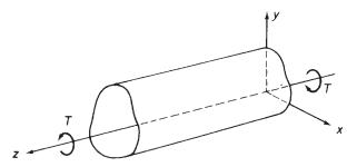
Fig. 18.1 Torsion of a closed section beam.
