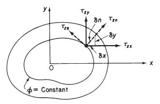
Fig. 3.5 Lines of shear stress.
