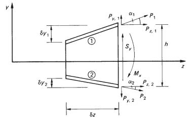
Fig. 21.1 Effect of taper on beam analysis.
