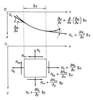
Fig. 7.12 In-plane forces on plate element.
