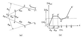
Fig. 27.8 Computation of torsion bending constant  $\Gamma_R$ : (a) dimensions of flat-sided open section beam; (b) variation of 2A<sub>R,0</sub> around beam section.
