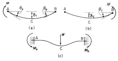
Fig. 5.28 Model analysis of a fixed beam.
