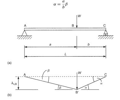
Fig. 4.8 Determination of bending moment at a point in the beam of Example 4.2 using virtual work.
