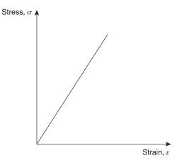
Fig. 11.16 Stress-strain curve for a fibre composite.
