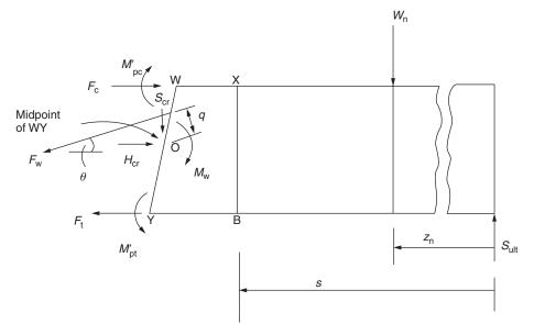
Fig. 9.19 Determination of flange forces.
