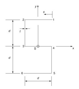
Fig. 8.19 Section of column of Example 8.5.
