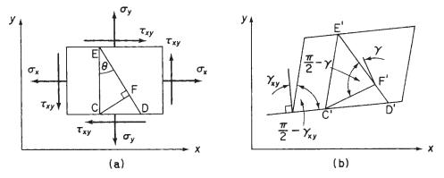
Fig. 1.16 (a) Stress system on rectangular element; (b) distorted shape of element due to stress system in (a).
