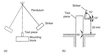
Fig. 11.7 Izod impact test.
