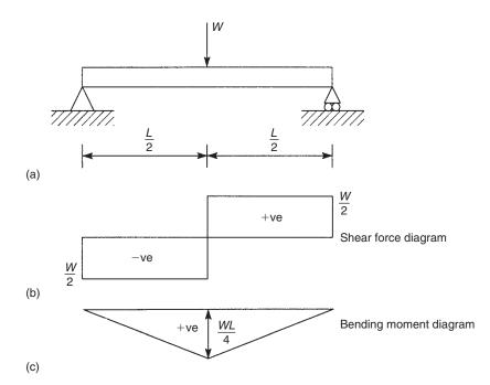
Fig. 11.4 Bending test on a beam, single load.
