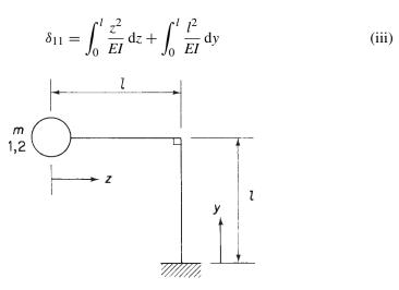
Fig. 10.7 Mass/beam system for Example 10.3.
