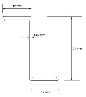
Fig. A.10 Stringer section, AA to CC (Type A).
