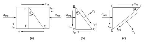
Fig. 9.16 Determination of stresses on planes parallel and perpendicular to the plane of the buckle.
