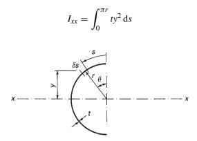
Fig. 16.33 Second moment of area of a semicircular section.
