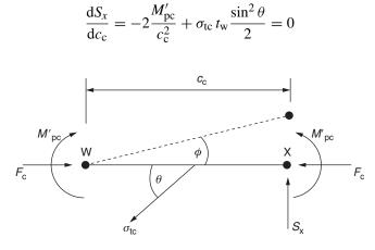
Fig. 9.17 Determination of plastic hinge position.
