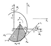
Fig. 27.18 Cross-section of an open section beam subjected to a general system of loads.
