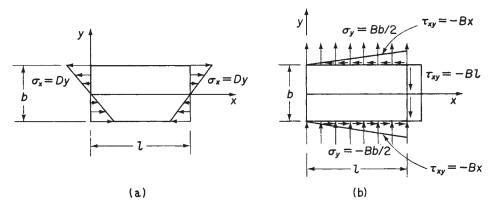
**Fig. 2.2** (a) Required loading conditions on rectangular sheet in Example 2.2 for A = B = C = 0; (b) as in (a) but A = C = D = 0.
