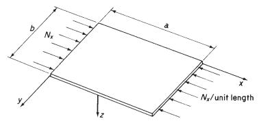
Fig. 9.1 Buckling of a thin flat plate.
