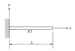
Fig. 10.12 Cantilever beam of Example 10.5.
