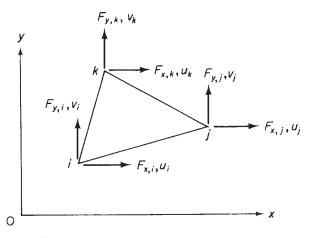
Fig. 6.13 Triangular element for plane elasticity problems.
