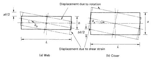
Fig. 18.9 Displacements due to twist and shear strain.
