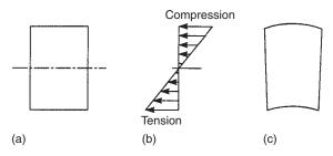
Fig. 16.8 Anticlastic bending of a beam section.
