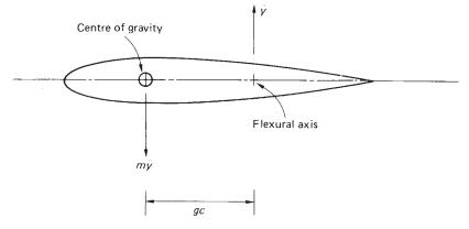
Fig. 28.8 Inertial coupling of a wing.
