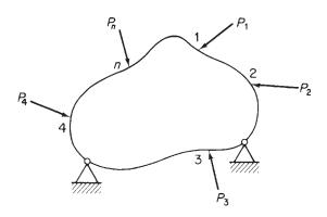
Fig. 5.26 Linearly elastic body subjected to loads P<sub>1</sub>, P<sub>2</sub>, P<sub>3</sub>, ..., P<sub>n</sub>.
