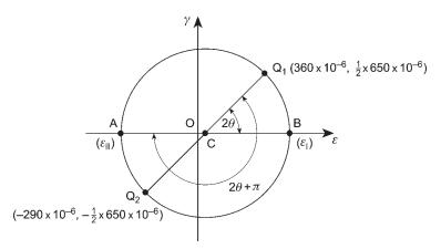
Fig. 1.17 Mohr's circle of strain for Example 1.5.
