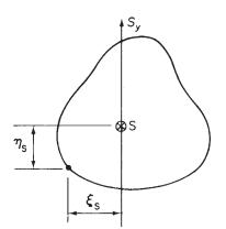
Fig. 17.12 Shear centre of a closed section beam.
