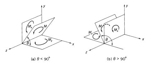
Fig. 16.11 Resolution of bending moments.
