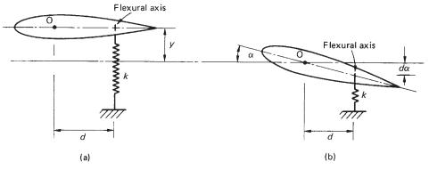
Fig. 28.9 Elastic coupling of a wing.
