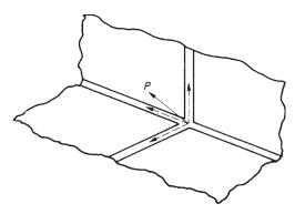
Fig. 24.6 Structural arrangement for an out of plane load.
