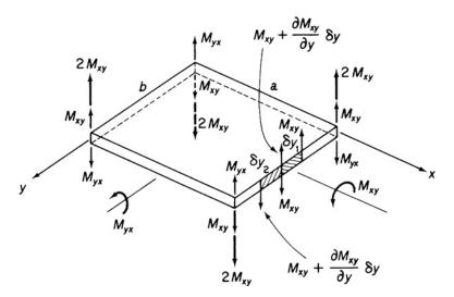
Fig. 7.11 Equivalent vertical force system.
