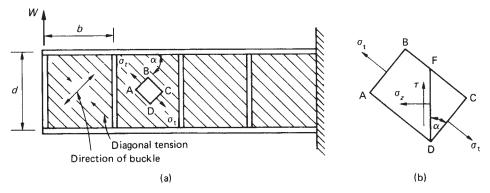
Fig. 9.8 Diagonal tension field beam.
