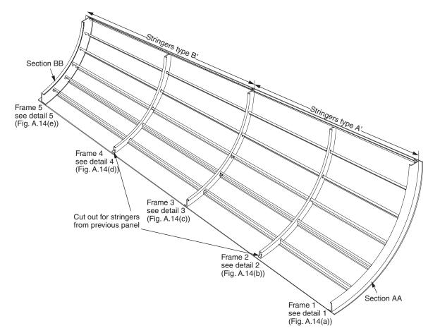
Fig. A.13 Layout of quarter fuselage.
