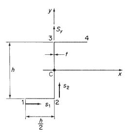
Fig. 17.6 Shear loaded Z-section of Example 17.1.
