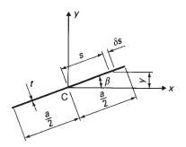
Fig. 16.32 Second moments of area of an inclined thin section.
