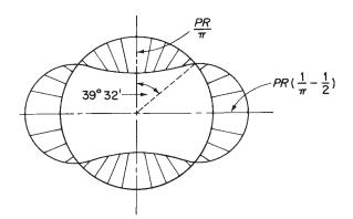
Fig. 5.15 Distribution of bending moment in a doubly symmetric ring.
