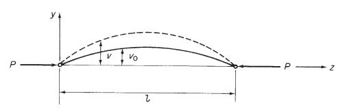
Fig. 8.9 Initially bent column.
