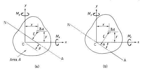
Fig. 16.12 Determination of neutral axis position and direct stress due to bending.
