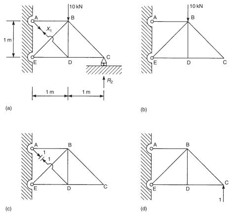
Fig. 5.21 Statically indeterminate truss of Example 5.9.
