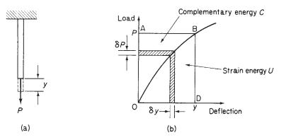
Fig. 5.1 (a) Strain energy of a member subjected to simple tension; (b) load–deflection curve for a nonlinearly elastic member.
