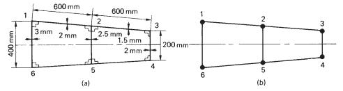
Fig. 20.4 Idealization of a wing section.
