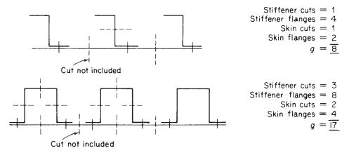
Fig. 9.7 Determination of *g* for two types of stiffener/skin combination.
