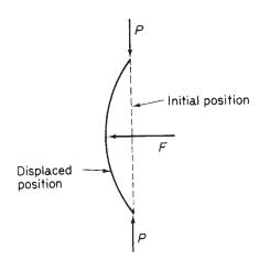
Fig. 8.1 Definition of buckling load for a perfect column.
