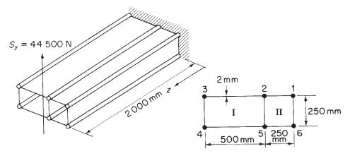
Fig. 23.15 Deflection of two-cell wing section.
