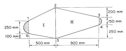
**P.23.3** Determine the torsional stiffness of the four-cell wing section shown in Fig. P.23.3.
