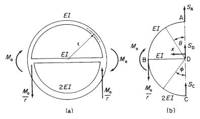
Fig. 5.17 Determination of bending moment distribution in an antisymmetrical fuselage frame.
