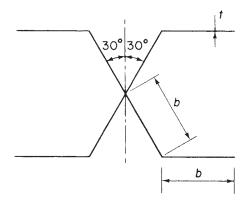
**P.8.16** A pin-ended column of length 1.0 m has the cross-section shown in Fig. P.8.16. If the ends of the column are free to warp determine the lowest value of axial load which will cause the column to buckle, and specify the mode. Take  $E = 70\,000\,\text{N/mm}^2$  and  $G = 25\,000\,\text{N/mm}^2$ .
