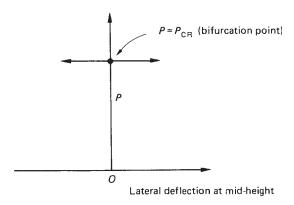
Fig. 8.4 Behaviour of a perfect pin-ended column.
