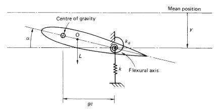
Fig. 28.10 Flutter of a wing section.
