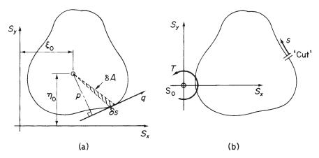
**Fig. 17.11** (a) Determination of  $q_{s,0}$ ; (b) equivalent loading on 'open' section beam.
