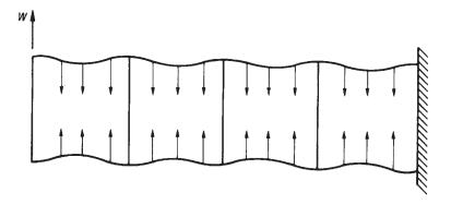
Fig. 9.11 Bending of flanges due to web stress.
