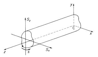
Fig. 17.10 Shear of closed section beams.
