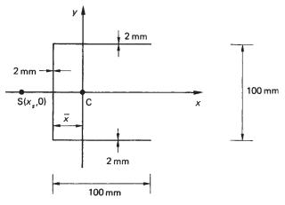
Fig. 8.18 Column section of Example 8.4.
