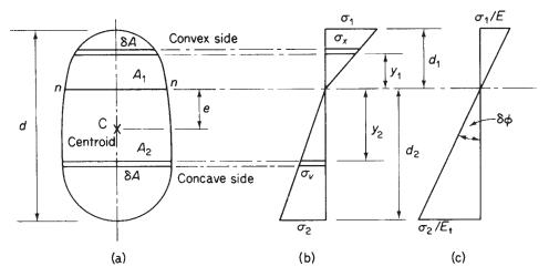
Fig. 8.8 Determination of reduced elastic modulus.
