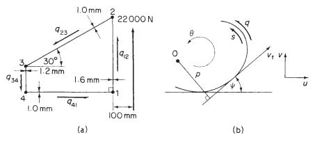
Fig. 26.2 (a) Beam cross-section at built-in end; (b) notation and sign convention.
