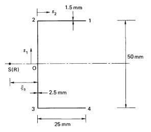
Fig. 18.12 Channel section of Example 18.3.
