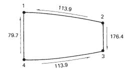
Fig. 23.27 Shear flows (N/mm) applied to the wing rib at station 3000 in the wing box of Example 23.7.
