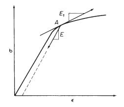
Fig. 8.7 Elastic moduli for a material stressed above the elastic limit.
