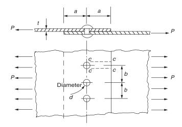
Fig. 12.11 Simple riveted lap joint.
