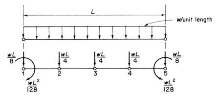
Fig. 6.8 Idealization of a beam supporting a uniformly distributed load.
