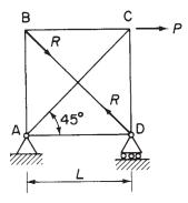
Fig. 5.8 Analysis of a statically indeterminate framework by the method of complementary energy.
