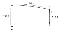
Fig. 23.24 Final shear flows (N/mm) in the cut-out bay of the wing box of Example 23.7.
