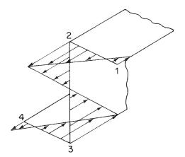
Fig. 16.35 Distribution of direct stress in Z-section beam of Example 16.14.
