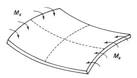
Fig. 7.3 Anticlastic bending.
