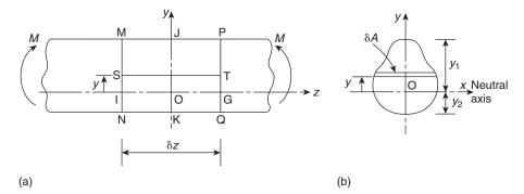
Fig. 16.4 Bending of a symmetrical section beam.
