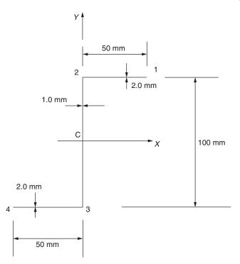
Fig. 25.11 Beam section of Example 25.5.
