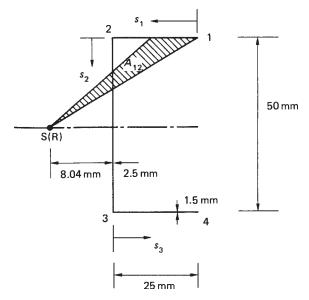
Fig. 18.14 Determination of points of zero warping.
