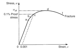
Fig. 11.13 Stress-strain curve for aluminium.
