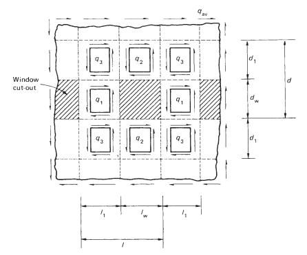
Fig. 22.5 Fuselage panel with windows.
