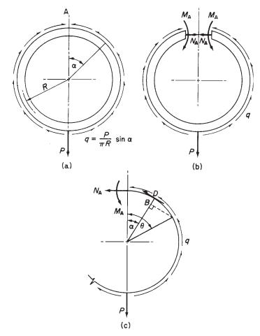
Fig. 5.16 Determination of bending moment distribution in a shear and direct loaded ring.
