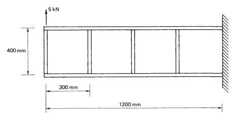
Fig. 9.12 Beam of Example 9.1.
