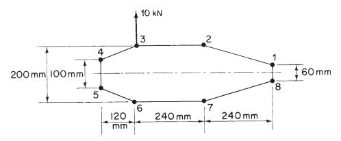
Fig. 20.11 Closed section of beam of Example 20.4.
