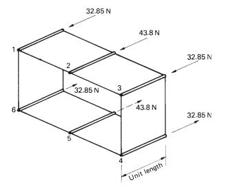
Fig. 21.9 Change in boom loads/unit length of beam.
