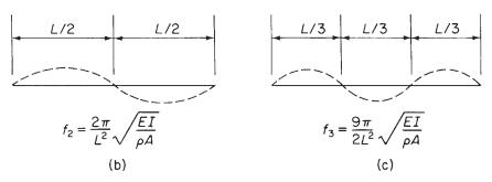
Fig. 10.11 First three normal modes of vibration of the beam of Example 10.4.
