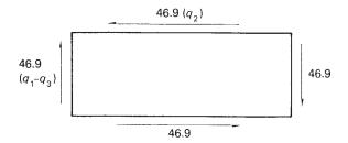
Fig. 23.20 Shear flows (N/mm) on wing rib at station 3000 in the wing of Example 23.6.
