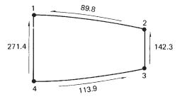
**Fig. 23.26** Final shear flows in bay 3 (and bay 1) of the wing box of Example 23.7.
