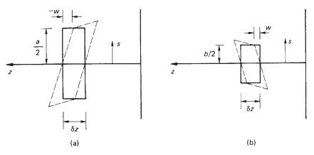
Fig. 26.7 Shear distortion of (a) an element of the top cover; (b) an element of the right hand web.
