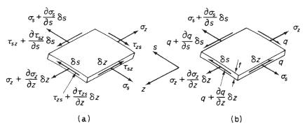
Fig. 17.1 (a) General stress system on element of a closed or open section beam; (b) direct stress and shear flow system on the element.
