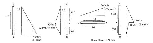
Fig. 24.5 Load distributions in stiffeners of the beam of Example 24.1.
