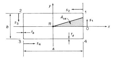
Fig. 18.4 Torsion of a rectangular section beam.
