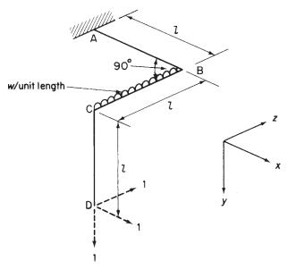
Fig. 5.19 Deflection of a bent rod.
