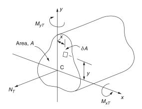
Fig. 16.36 Beam section subjected to a temperature rise.
