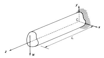
Fig. 16.24 Determination of the deflection of a cantilever.
