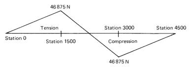
Fig. 23.19 Distribution of load in the top flange of the front spar of the wing of Example 23.6.
