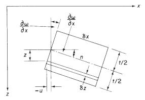
**Fig. 7.7** Determination of shear strain  $\gamma_{XY}$ .
