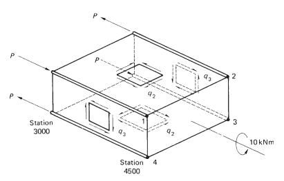
Fig. 23.18 Loads on bay ③ of the wing of Example 23.6.
