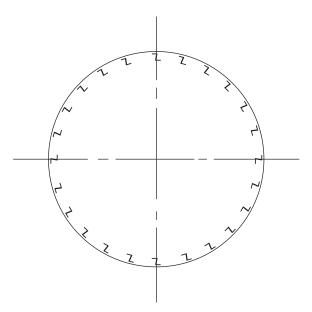
Fig. A.5 Stringer arrangement in rear fuselage.
