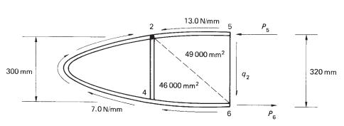
Fig. 24.11 Equilibrium of rib forward of intermediate stiffener 56.
