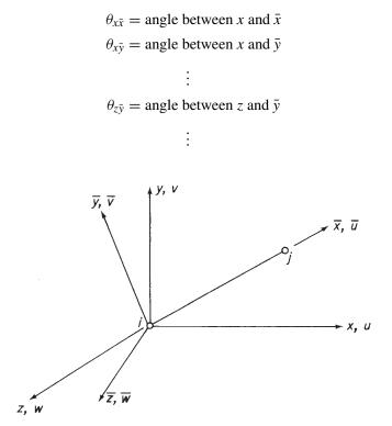
Fig. 6.5 Local and global coordinate systems for a member in a pin-jointed space frame.
