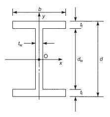
Fig. 16.28 Second moments of area of an I-Section.
