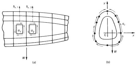
Fig. 24.8 Loads on a fuselage frame.
