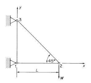
Fig. 6.4 Pin-jointed framework of Example 6.1.
