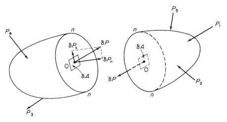
Fig. 1.2 Internal force components at the point O.
