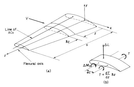
Fig. 28.3 Determination of wing divergence speed (three-dimensional case).
