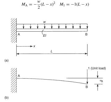
Fig. 4.10 Deflection of the free end of a cantilever beam using the unit load method.
