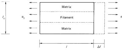
Fig. 25.1 Determination of E<sub>I</sub>.
