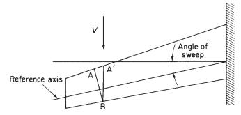
Fig. 28.4 Effect of wing sweep on wing divergence speed.
