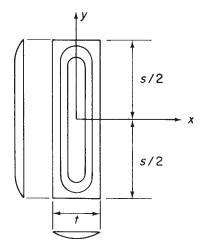
Fig. 3.9 Torsion of a narrow rectangular strip.
