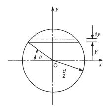
Fig. 16.29 Second moments of area of a circular section.
