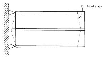
Fig. 26.19 Displaced shape of top cover of box team of Fig. 26.18.
