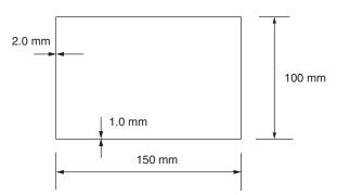
**P.25.3** If the thin-walled box beam of Fig. P.25.2 carries a bending moment of 1 kN m applied in a vertical plane, determine the maximum direct stress in the cross-section of the beam.
