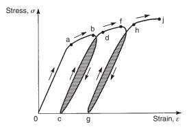
Fig. 11.17 Strain hardening of a material.
