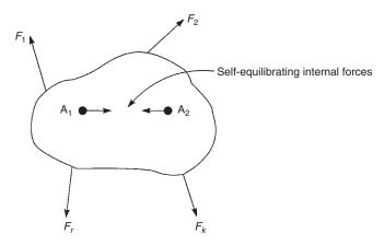
Fig. 4.3 Virtual work for a rigid body.
