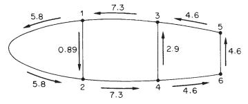
Fig. 23.7 Shear stress (N/mm<sup>2</sup>) distribution in wing section of Example 23.2.
