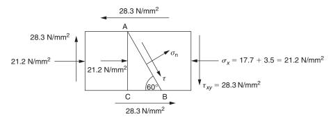
Fig. 1.11 Stress system on two-dimensional element of the beam of Example 1.2.
