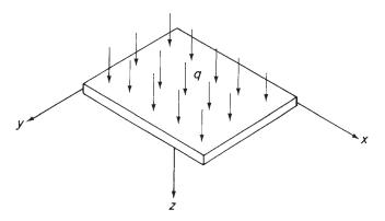
Fig. 7.8 Plate supporting a distributed transverse load.
