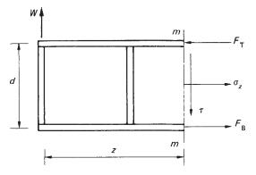
Fig. 9.9 Determination of flange forces.
