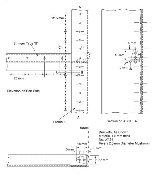
Skins from Previous Sections Overlap Where Necessary Rivets 2.5 mm Diameter Countersunk.
