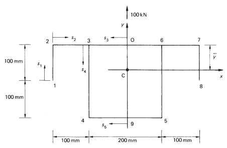
Fig. 19.2 Beam section of Example 19.1.
