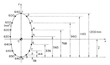
Fig. 20.5 Idealized fuselage section of Example 20.2.
