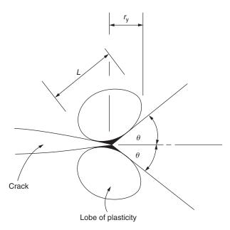
Fig. 15.6 Plane strain plasticity.
