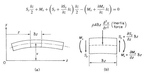
Fig. 10.9 Vibration of a beam possessing mass.
