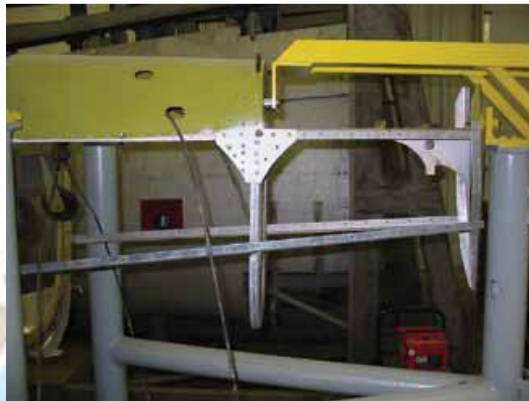
Gussets are used to increase strength.
