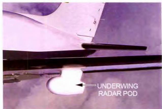
Radar antenna for a single-engine airplane cannot mount in the nose because of the propellor. Instead, it is located under the wing, as shown above, or built into the leading edge of wing.
