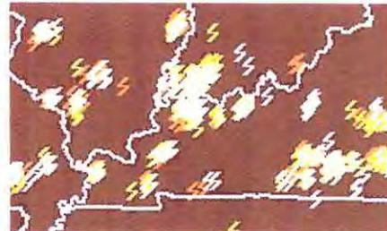
Lightning strikes measured from the ground by the National Lightning Detection Network are updated every five minutes and sent to the aircraft by datalink.
