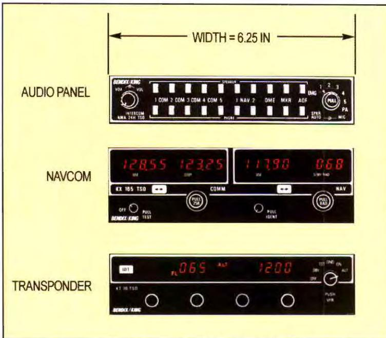
Radios in the center stack of a light aircraft are usually 6.25 inches wide.
