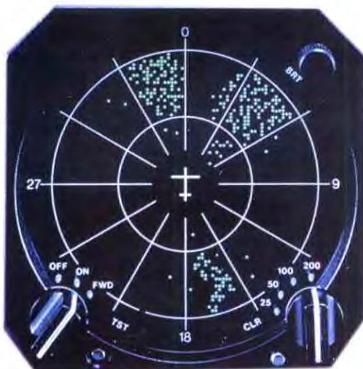
The Stormscope shows each lightning stroke as a green dot. The three large dot clusters are groups of thunderstorm cells. The display is 360 degrees, with the airplane in the center, thus showing activity behind the airplane. If the pilot wants to avoid storms ahead, he'll know not to make a 180-degree turn and fly into more storms.
