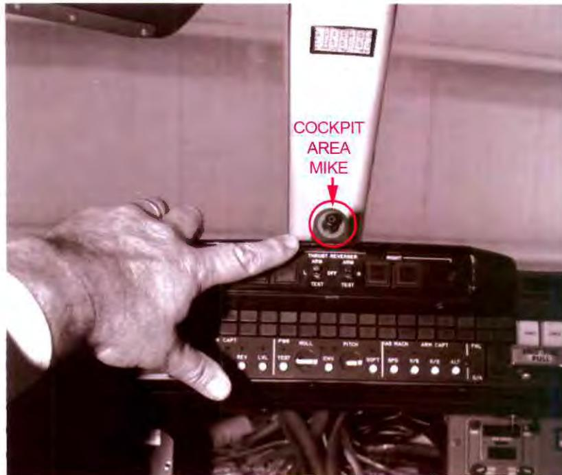
Cockpit area microphone picks up conversation between pilots and other sounds that provide clues for accident investigators. This mike is located atop the glareshield on a small corporate jet. In airliners, the mike is usually above, on the overhead panel.
