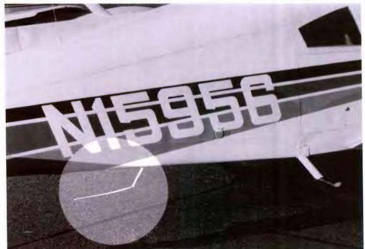
When a com antenna must be mounted on the belly of a light aircraft, use a "bent whip" to prevent striking the ground. Although not as efficient as a top-mounted antenna, the bent whip shown here was used for 10 years. It reliably communicated 50 miles in every direction at an altitude of 3000 feet,
