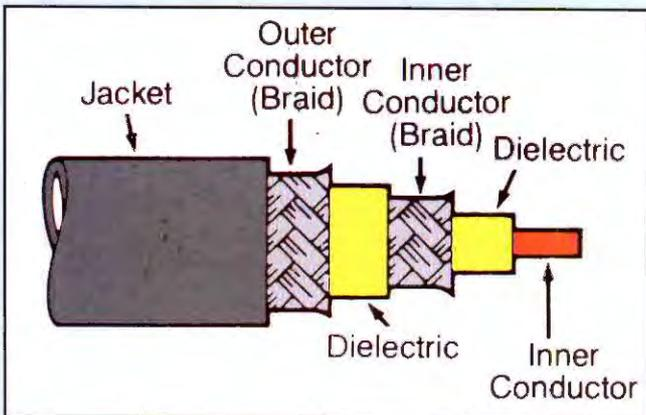
Triaxial cable, with two outer conductors separated by insulation. The outer conductor (braid) serves as a signal ground, while the other is an earth ground. This arrangement provides very high immunity to electrical noise.
