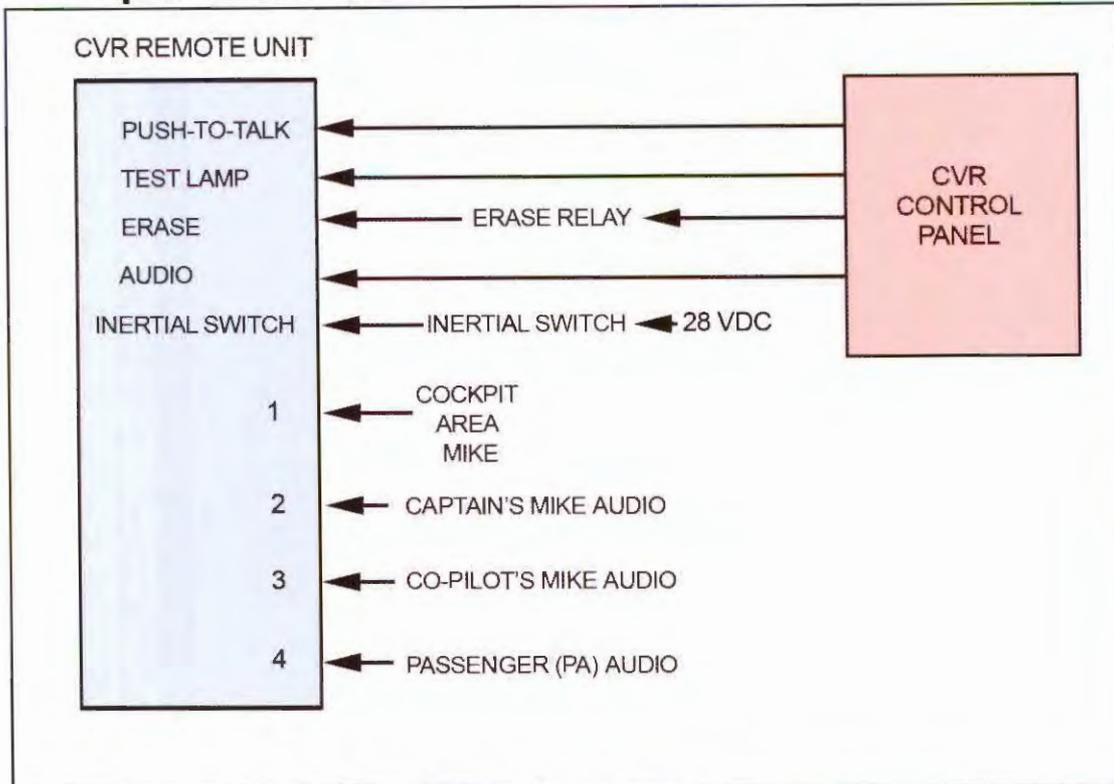
Line Replaceable Unit, at left, is mounted in the aft fuselage in a crash-hardened housing. It records four audio channels; captain's mike, co-pilot's mike, cockpit area mike and public address. Test and erase functions are done at the controller on the instrument panel (right).
