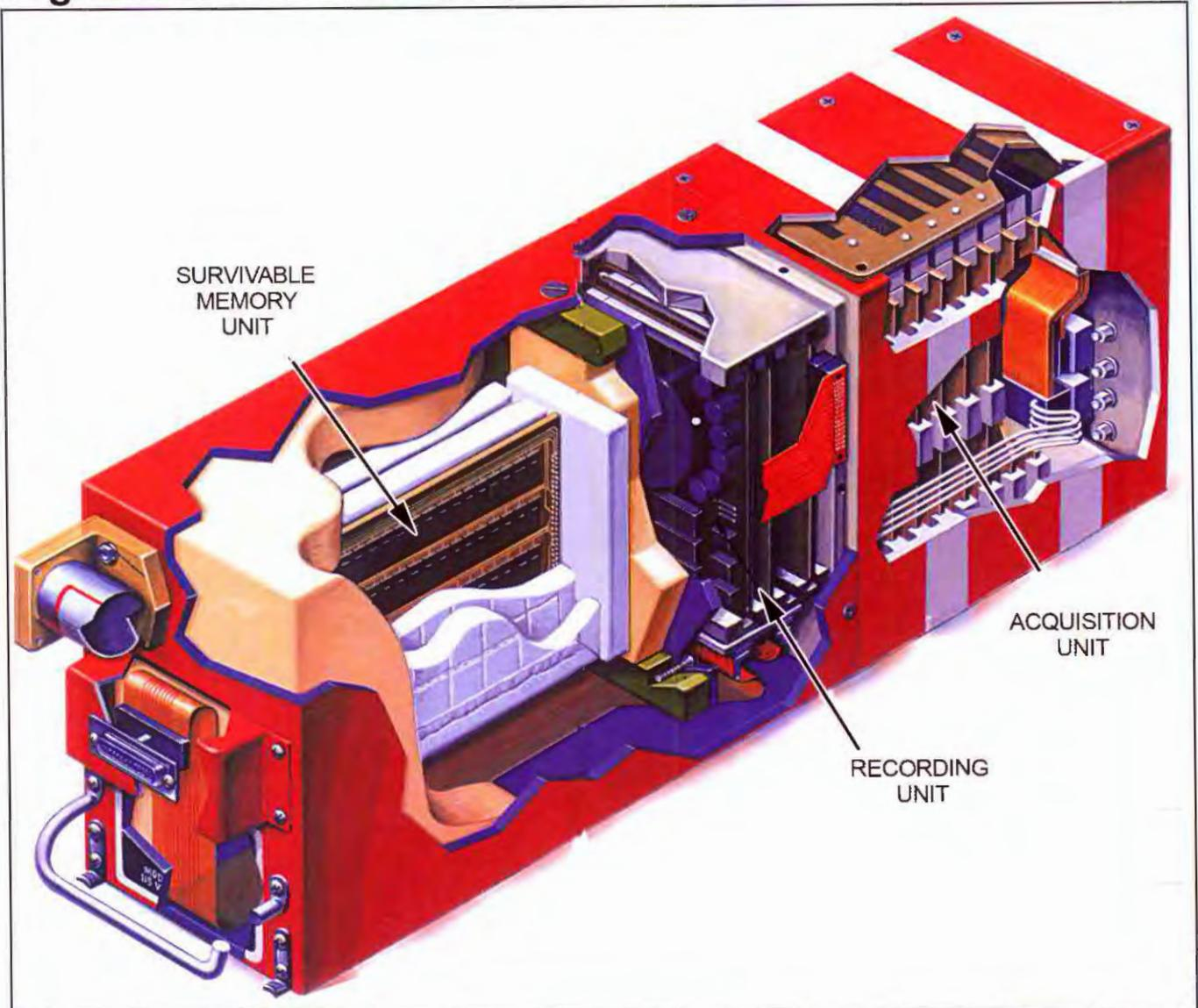
Solid-State Flight Data Recorder (SSFDR) by Lockheed eliminates tape storage with a survivable solid-state memory. It is interchangeable with earlier-generation recorders without wiring changes.
