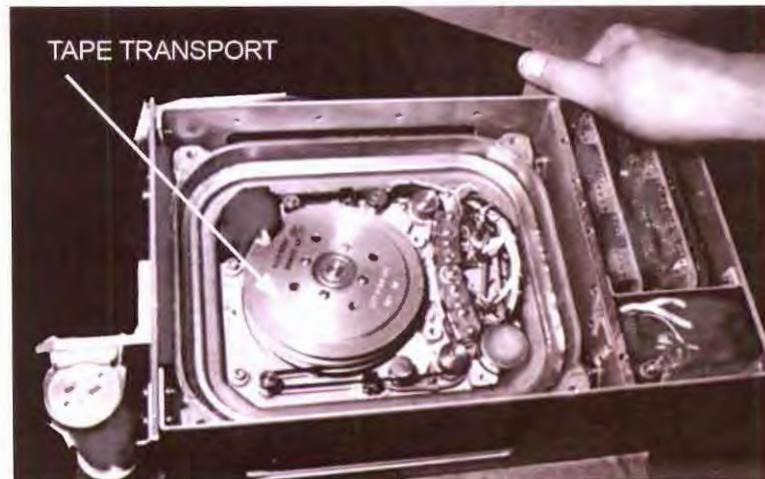
Early cockpit voice recorders use a tape and mechanical drive. Next-generation recorders eliminate tape with more reliable solid-state memory. New recorders meet tougher requirements for heat and G-forces and need less maintenance.
