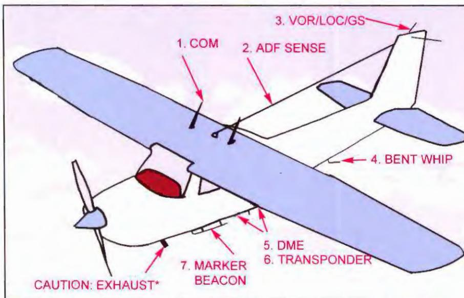
Don't locate an antenna on the belly in centerline of the fuselage, but avoid cutting into structure like ribs and stringers.
