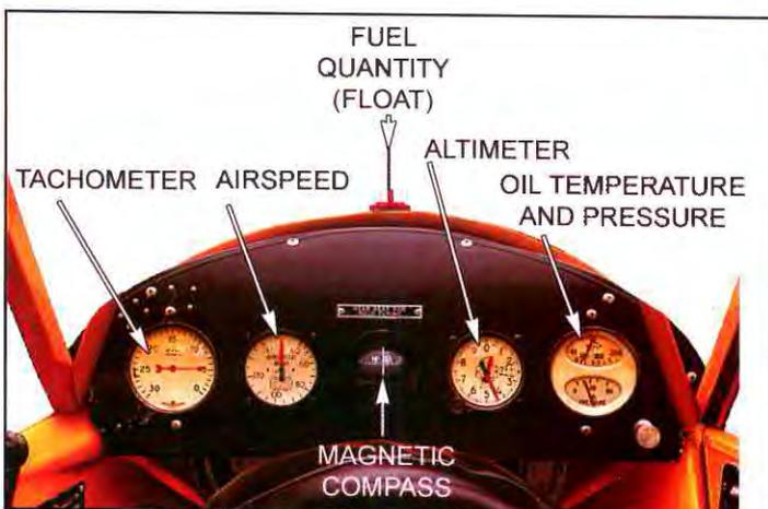
Instrument panel of the original Piper Cub, which received its Type Certificate in 1931. Today, the same instruments are still required for “day VFR” flying. More airplanes, however, show the same information on an electronic display, as seen on the next page.
