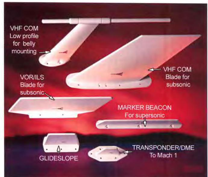
**Antennas by HR Smith for high-performance aircraft are encased in thermosplastic composite material to resist rain erosion, impact, chemicals and temperature changes.**
