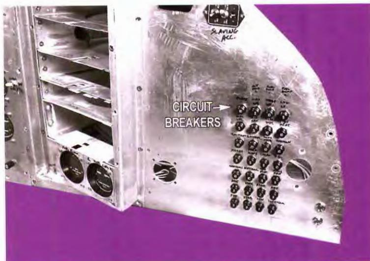
Circuit breakers during construction of a panel Note that each breaker is temporarily labelled with a felt-tip pen. This helps identify the wiring and final testing. After the panel is painted, machine-made labels are applied.
