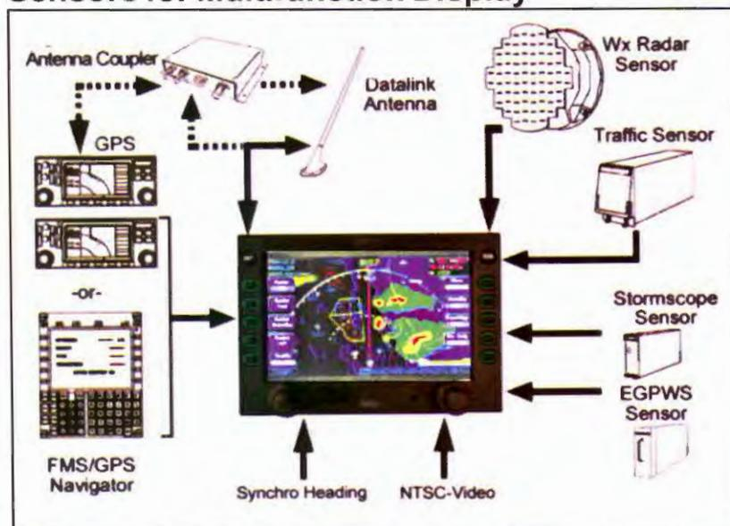
Many sensor and data inputs are required to drive the MFD. The system has standard industry interfaces (such as ARINC 429 and IEEE RS-232), as well as interfaces to accept signals from other manufacturers' products for radar, lightning, terrain and traffic information.
