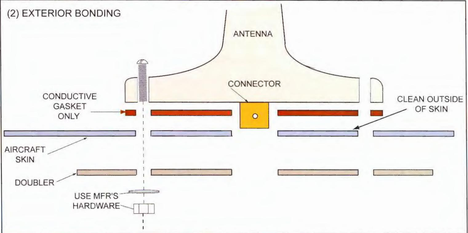
In the exterior method, bonding is made to the outside skin. Thus, the skin must be cleaned and treated with Alodine to prevent corrosion. Only a *conductive* gasket can be used with exterior bonding; there must be good electrical contact with the outer skin.
