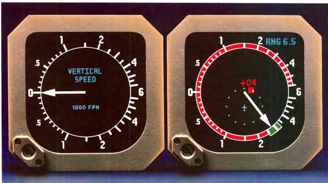
Aircraft without electronic flight instruments (EFIS) may add a TCAS display by replacing the conventional VSI (vertical speed indicator) shown at the left.
