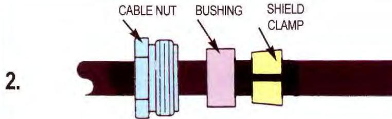
Slide the hardware (cable nut, bushing and shield clamp) over the cable
