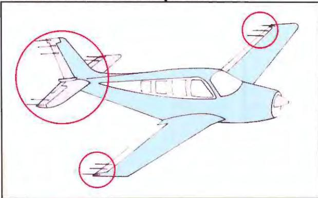
Typical locations are shown for static wicks on trailing edges of wings and tail. Manufacturers of wicks provide drawings for most aircraft that show exact locations.
