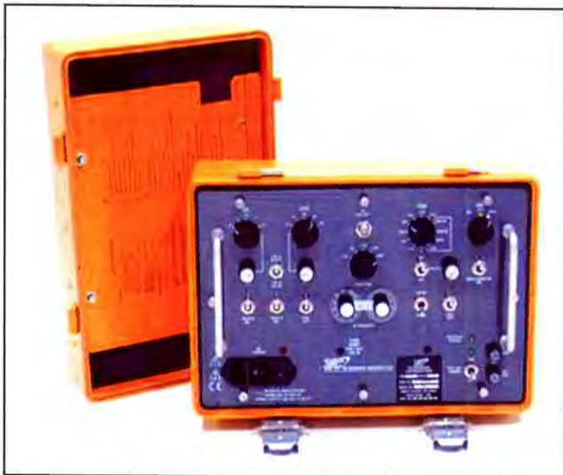
Ramp test set for checking a Category III ILS aircraft receiver. It generates a variety of signals such as VOR, glideslope, localizer, and marker beacon, as well as autopilot and flight director. The tester is operated by one person in the cockpit while the aircraft is on the ground. Shown here is the Model T-30D by TIC.
