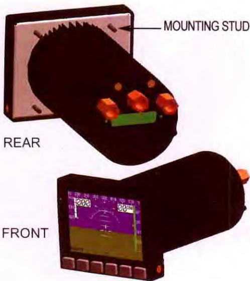
Some instrument cases are fitted with mounting studs, as in this Dynon EFIS display. Four holes are drilled in the instrument panel according to the template (below) supplied by the manufacturer. The large hole receives the instrument case.
