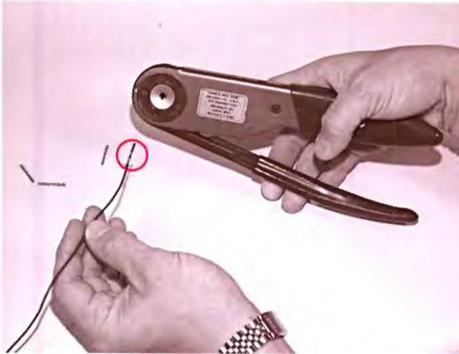
Connector contact (in red circle) is crimped to the end of a wire with a crimping tool (type DMC AF8).
