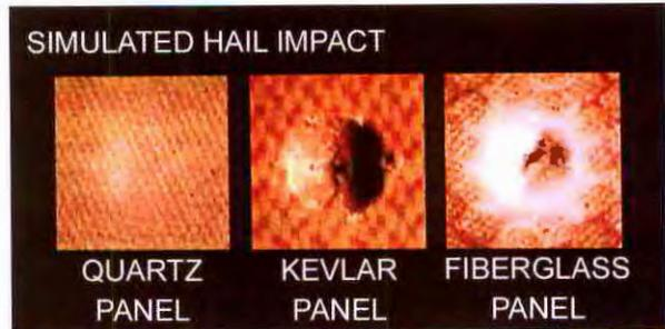
Radomes erode, especially in high-performance aircraft. The test shown above illustrates a radome constructed of quartz, which has proven light and strong compared to other materials.
