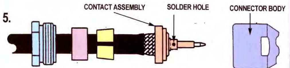
The contact assembly is pushed under the shield. Apply solder to the hole and heat just enough for solder to fuse with the wire and contact.
