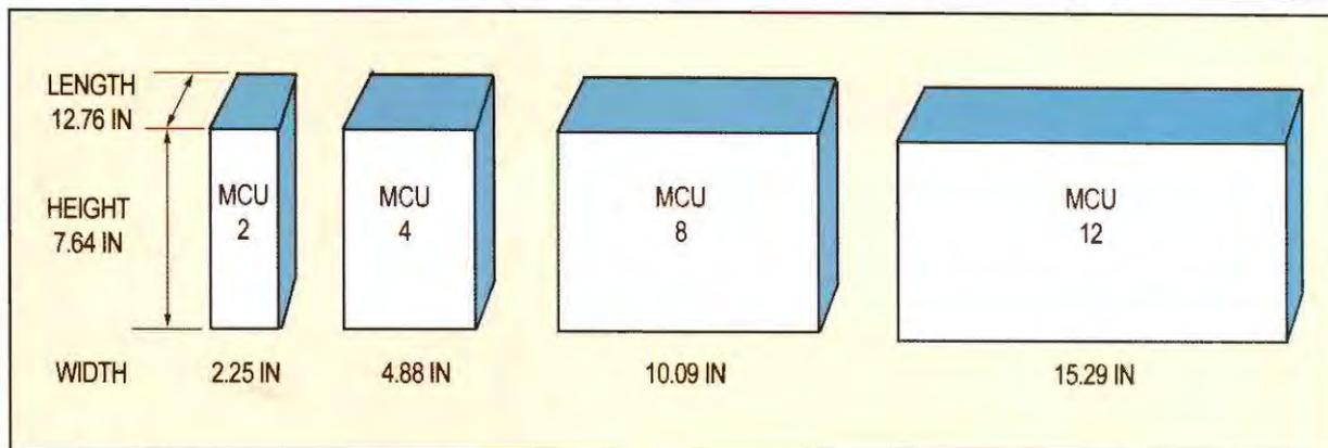
When airliners began converting to digital avionics, new case sizes were developed for LRU's (line replaceable units). Called MCU, for Modular Concept Unit, it was standardized by ARINC 600. The connectors offer many more circuits over ARINC 404. Because "digital airliners" still carry analog equipment, they have a mixture of ARINC 404 and 600 cases.
