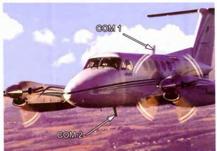
VHF com antennas are usually placed top and bottom, as in this King Air, when the aircraft is certified for flight in icing conditions. Ice on an antenna may cause vibration and breakage. It is unlikely that both top and bottom antennas will be affected the same way because of different slipstreams.
