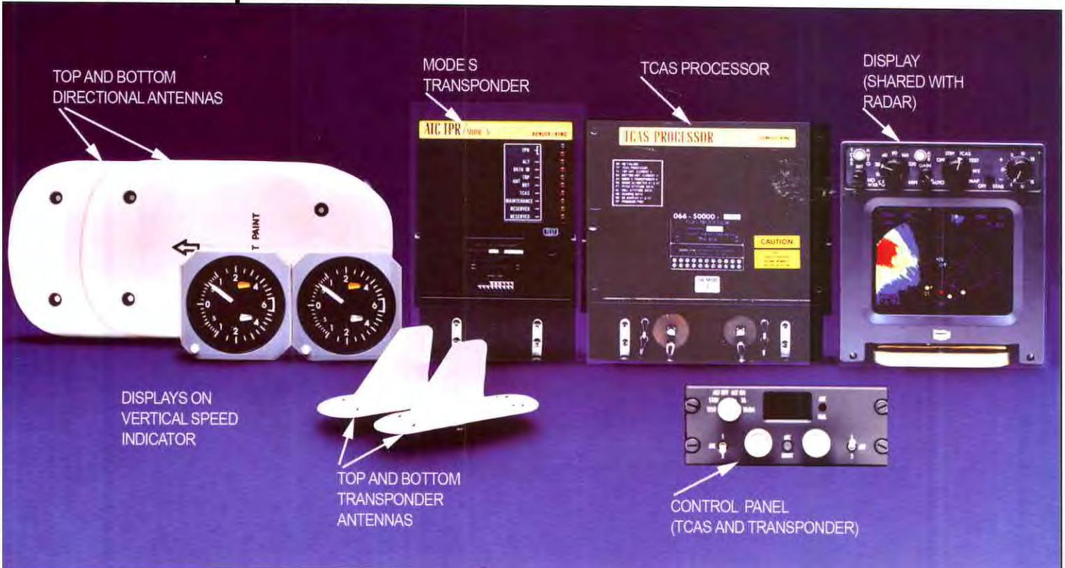
The control panel at lower right selects TCAS and transponder functions. Two antennas are used for the transponder---placed at top and bottom of the fuselage---to
