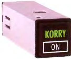
Improved lighted pushbutton switches, like this Korry model, eliminate a major source of maintenance; replacing lamps with burned-out filaments. Lighting is supplied by bright LED's (light emitting diodes) that can last the life of the airplane. They also run cooler than conventional lamps.
