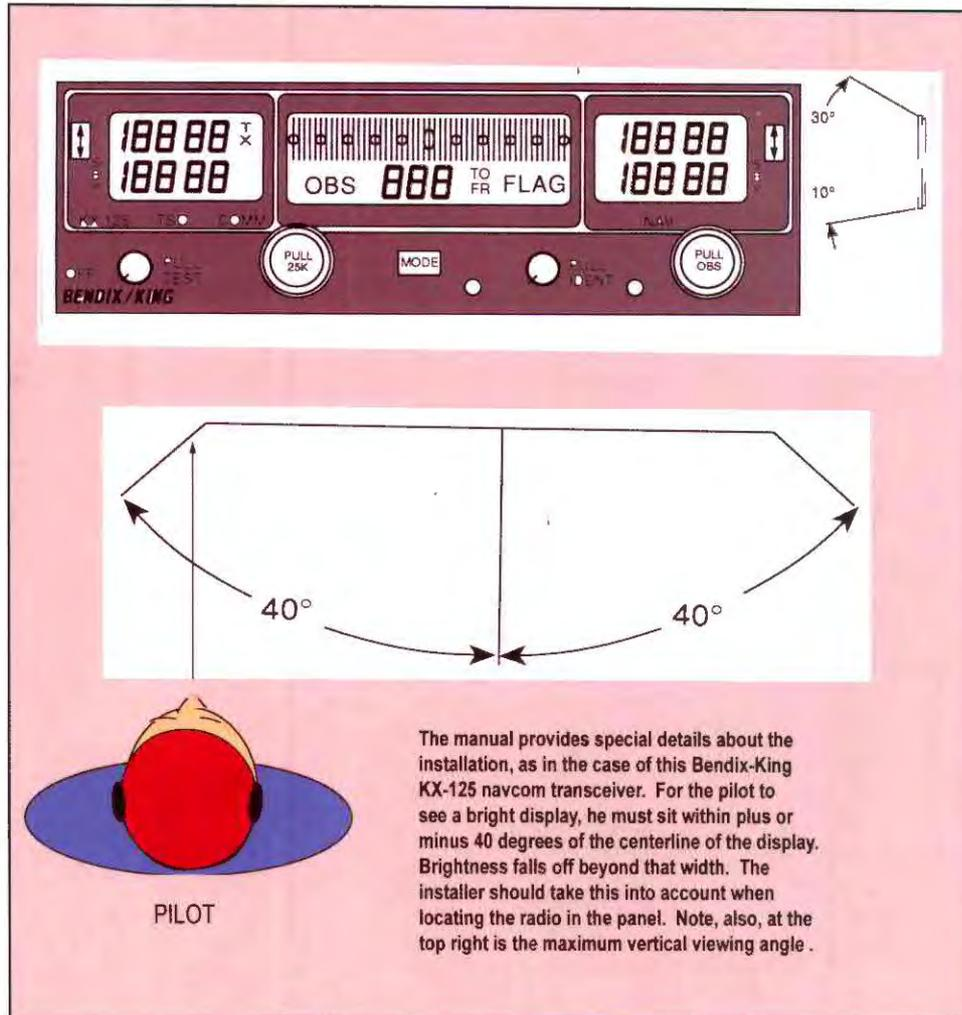
The diagram illustrates the viewing angle requirements for the Bendix-King KX-125 navcom transceiver. The top part shows the device with a 30-degree vertical viewing angle and a 10-degree horizontal viewing angle. The middle part shows a 40-degree horizontal viewing angle from the centerline. The bottom part shows a pilot's head and shoulders, labeled "PILOT".
