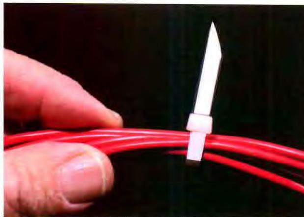
Cutting the tab too long and leaving a sharp point can injure the next person reaching for the harness under the instrument panel.
