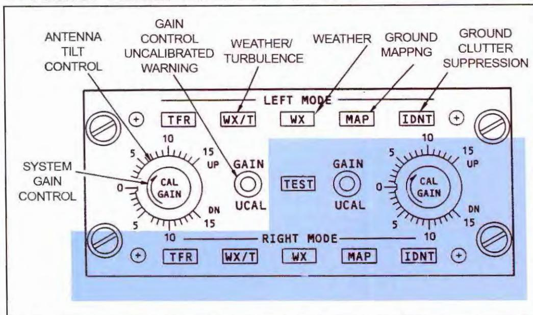
Both the captain and first officer operate the weather radar from the same control panel in this ARINC-type unit. Nearly all controls are duplicated; the captain's side is the white area, the co-pilot's is shown with a blue background. They are grouped as "Left Mode" and "Right Mode" to indicate that the controls affect left and right sides of the instrument panel.
