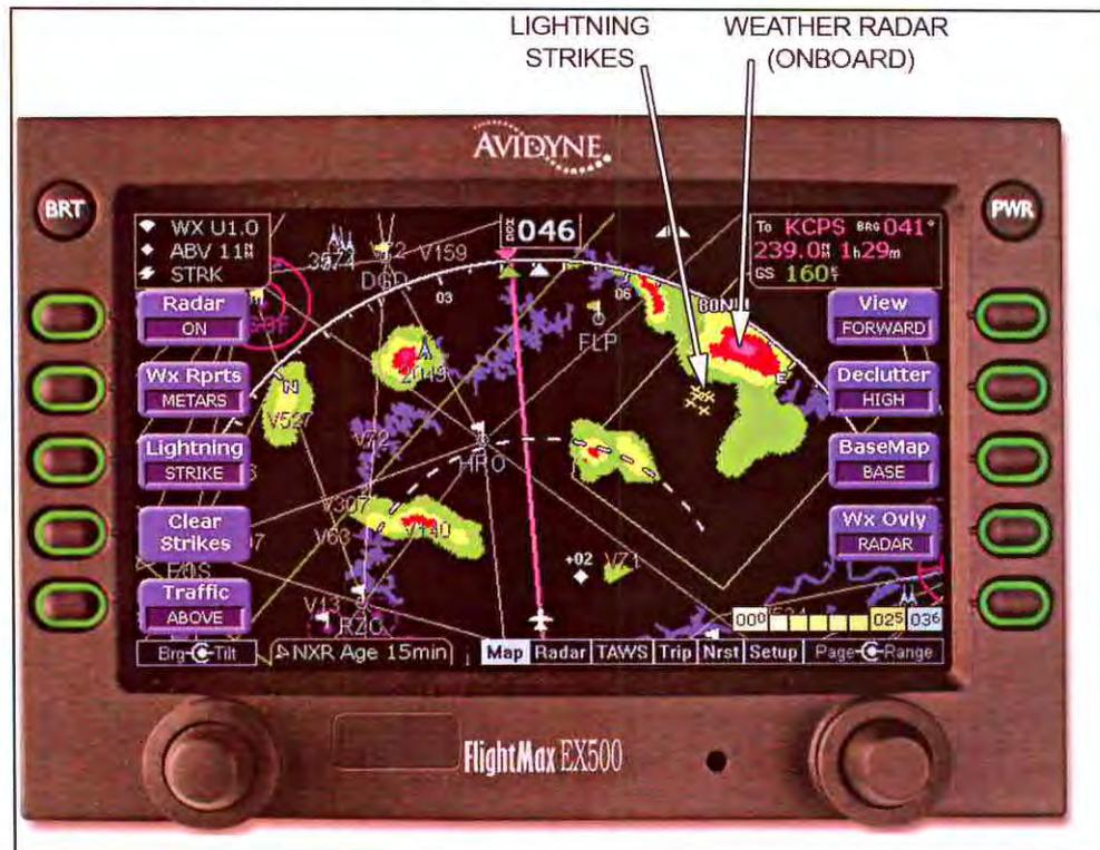
More aircraft are now outfitted with multifunction displays which overlay several sources on a basic moving map. This includes weather (rain or other precipitation) and lightning strikes. The information may be picked up by satellite or from an onboard radar or Stormscope.
