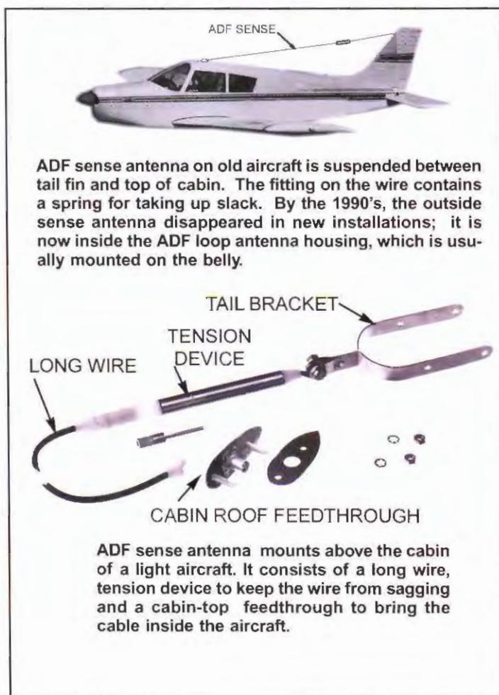
ADF sense antenna on old aircraft is suspended between tail fin and top of cabin. The fitting on the wire contains a spring for taking up slack. By the 1990's, the outside sense antenna disappeared in new installations; it is now inside the ADF loop antenna housing, which is usually mounted on the belly.
