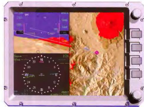
The old "radio stack" will disappear as new and upgraded airplanes, of even the smallest size, are outfitted with EFIS (Electronic Flight Instrument System). This Blue Mountain system combines flight instruments, moving map and terrain warning on one display.
