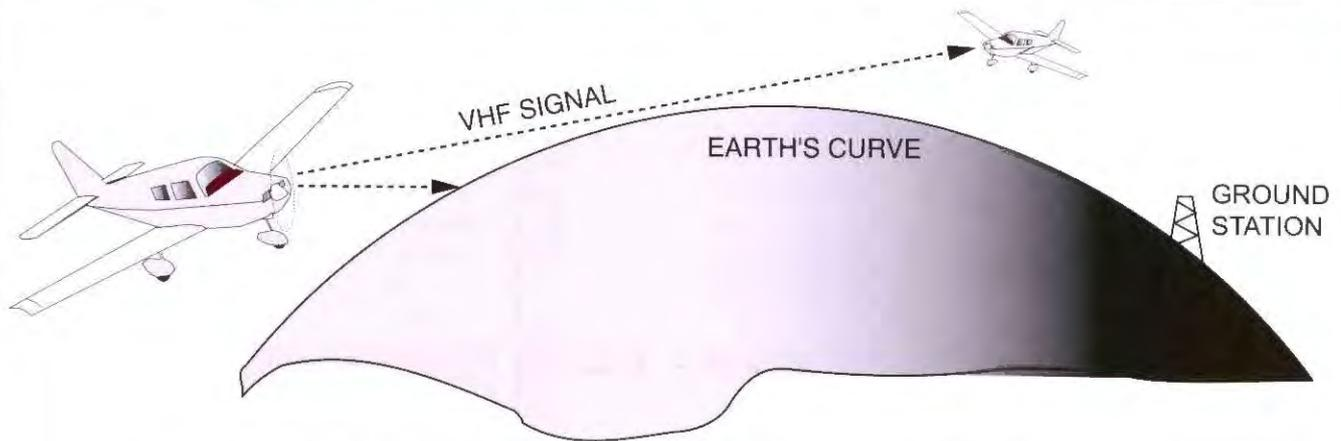
Signals in the VHF and higher bands travel in straight lines, with little effect from earth or ionosphere. This includes signals for VHF com and nav, GPS nav, transponder, DME, radar and other services above 30 MHz. Thus, the airplane at the left cannot communicate with the ground station on the far right because the signal is shaded by the earth. The two airplanes, however, can communicate because they "see" each other above the earth's horizon.
