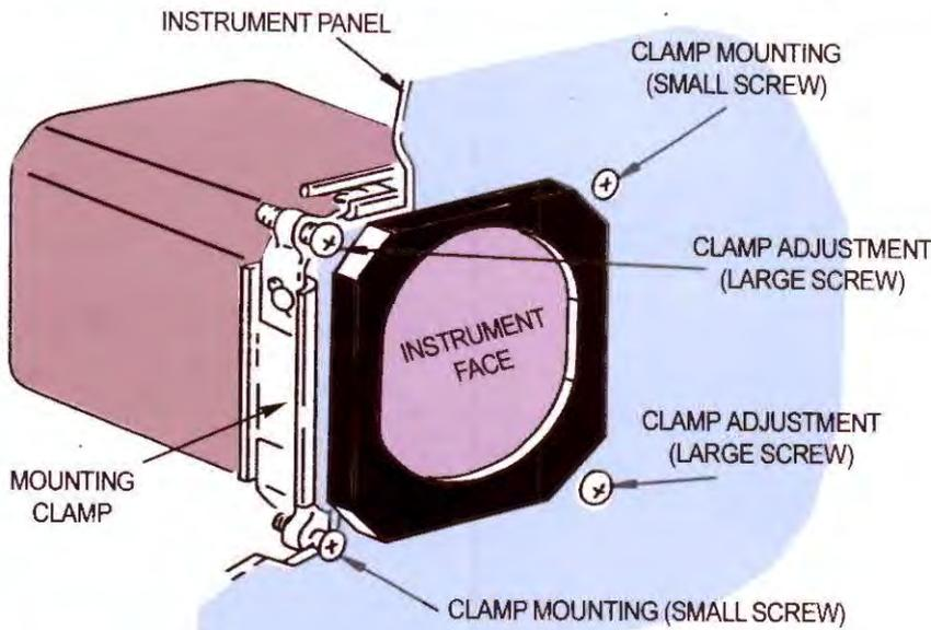
Instruments like this 3-inch rectangular are often held by a mounting clamp behind the panel. The clamp is slid over the case and two sets of screws are adjusted. Two screws have large heads labelled "Clamp Adjustment". They tighten the clamp around the case. The other pair, labelled "Clamp Mounting," hold the clamp to the back of the instrument panel.
