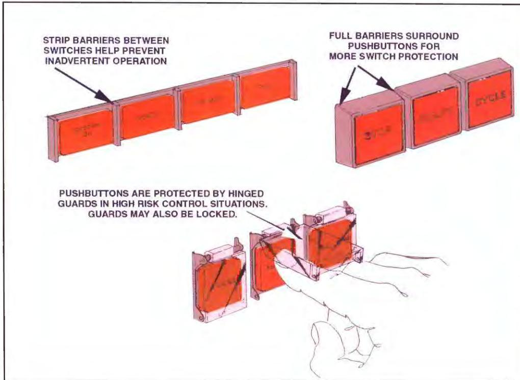
A pilot may push the wrong switch while flying in turbulence. Barriers between rows of switches reduce that problem. In the bottom drawing, switches are covered by a guard which must be lifted.
