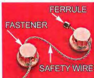
1. Pre-twisted safety wire is inserted into fasteners. A ferrule has been crimped to one end (upper right).
