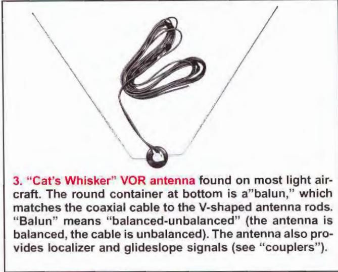
**3. "Cat's Whisker" VOR antenna** found on most light aircraft. The round container at bottom is a "balun," which matches the coaxial cable to the V-shaped antenna rods. "Balun" means "balanced-unbalanced" (the antenna is balanced, the cable is unbalanced). The antenna also provides localizer and glideslope signals (see "couplers").
