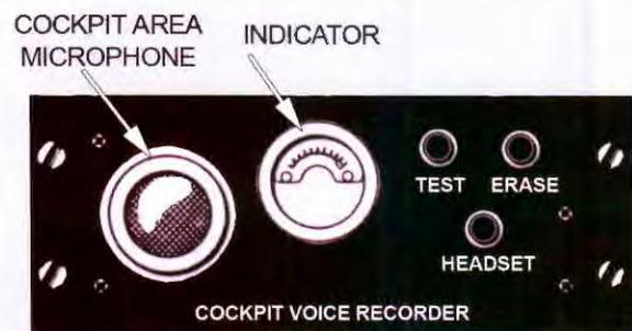
Controller for a cockpit voice recorder (early type). The cockpit area microphone picks up sound of pilot conversation, airplane, engine mechanical noises and warning tones.
