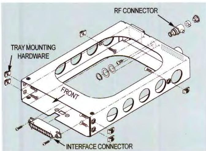
Preparing the tray for mounting. Hardware on the sides of the tray holds it to brackets in the instrument panel. The RF connector, which goes to an antenna, is fastened at the back. The interface connector will also mount on the rear of the tray, next to the RF connector. Holes along the sides of the tray lighten the structure.
