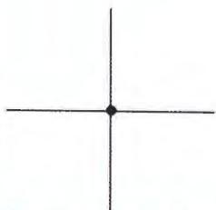
The dot indicates an electrical connection between the wires
