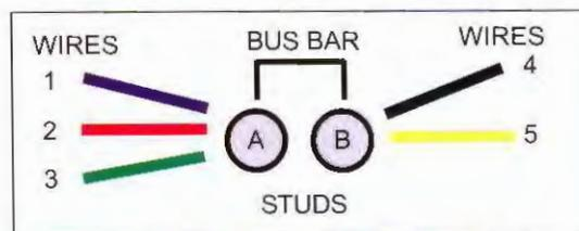
In this example, five wires must connect to one point. Three are connected "A". The bus bar, or jumper, connects "A" to "B". Up to three wires can connect to B without exceeding the limit of four connections per stud.
