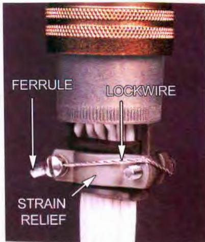
Strain relief for cable is provided by clamp at back of connector. Screws are secured by safety wire applied by tool.
