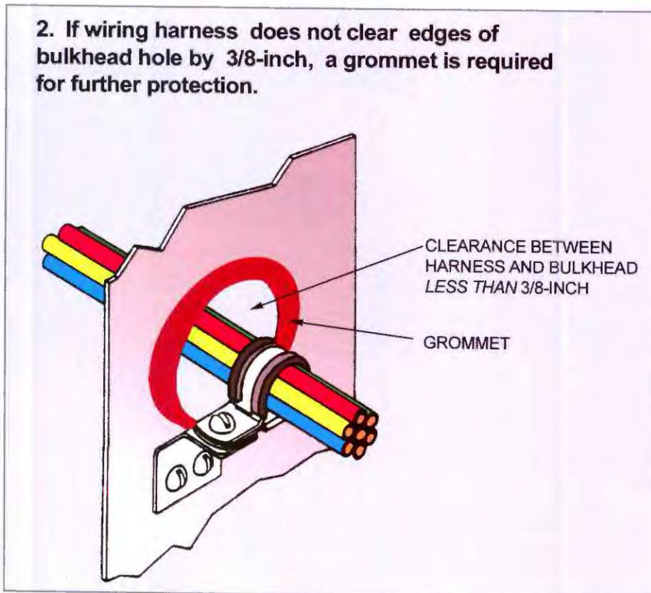
If there is less than 3/8-inch clearance, add a grommet to the hole. There are many openings in an airframe for running wire harnesses. They're known as "lightening holes" because they lighten the airframe. They are not "lightning" holes.
