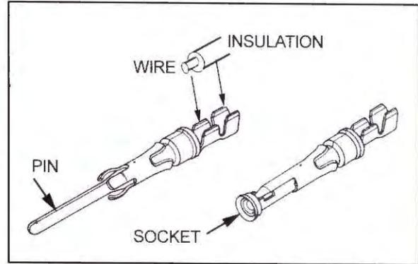
Pin and socket contacts that will be inserted into the connector. The wire is crimped into tabs on the contact. Another set of tabs clamps the insulation to relieve strain. These terminals are used in a "Molex" connector.
