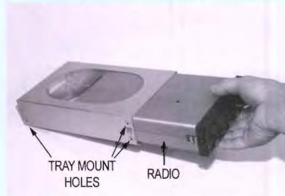
Radio is shown sliding into mounting tray. Holes in the tray are for fastening the tray to the instrument panel.
