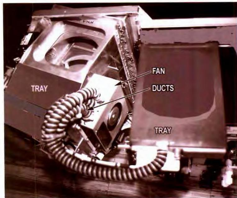
Behind the instrument panel of a light aircraft, showing cooling fan and ducts. The fan is attached to the side of the radio stack at the left. Several air ducts are seen emerging from the fan. They connect to ports on the radio trays, where they deliver cool air.
