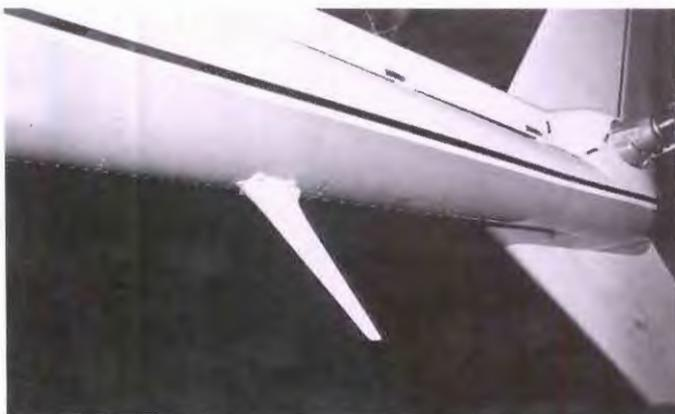
Com antenna on the bottom of a helicopter tail boom. Because of the main and tail rotor blades, antenna locations on helicopters are more difficult to find.
