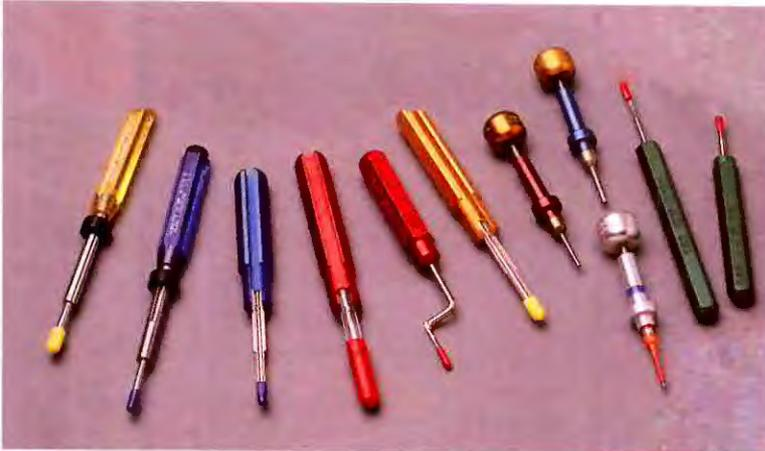
A variety of tools is available for installing and removing connector pins, either front or rear release. Although these tools may be offered in plastic, metal is preferred for durability.
