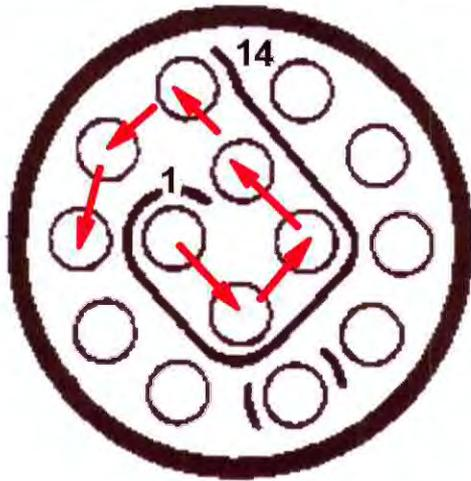
1. The end of a circular connector, where contacts will be inserted. Some connectors identify every contact, but limited space may allow only starting and ending numbers like "1" and "14," shown above. Start at "1" and follow the guide line around to "14," as shown by the arrows (which are not on the connector).
