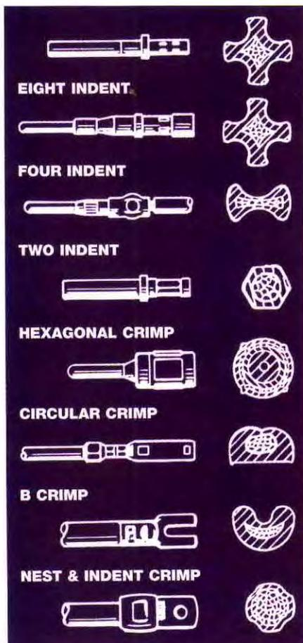
Crimp tools are fitted with dies <sup>DMC</sup> for making different crimp patterns. The most common for avionics work is the "Eight Indent" shown at the top.
