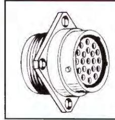
Circular connector with bayonet coupling.
