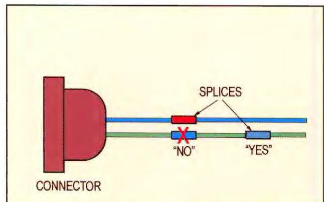
Each of the wires from this connector has a splice. Do not locate splices adjacent to each other. Stagger them to prevent overlapping, which causes bulges in the wire bundle that might not fit into tight spaces. Bulges also make future maintenance more difficult.
