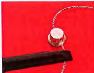
2. The other end of the wire is inserted into the tool nose, which stores ferrules.
