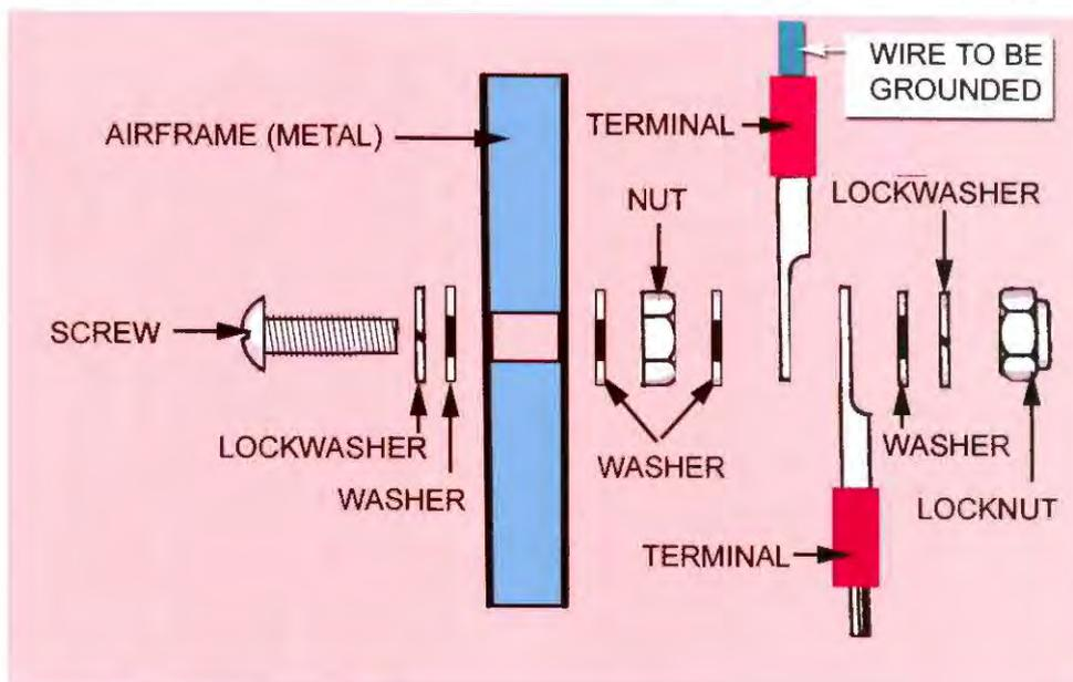
The procedure for attaching wires to the metal structure of the airplane. It serves one of two purposes. One is “grounding,” which provides a return connection to the power source for a radio or other electrical device. The whole airframe (if made of metal) is the return connection. The other is “bonding”, which connects two surfaces (flaps and wing, for example) with the lowest possible electrical resistance. This reduces the chance of generating interference.
