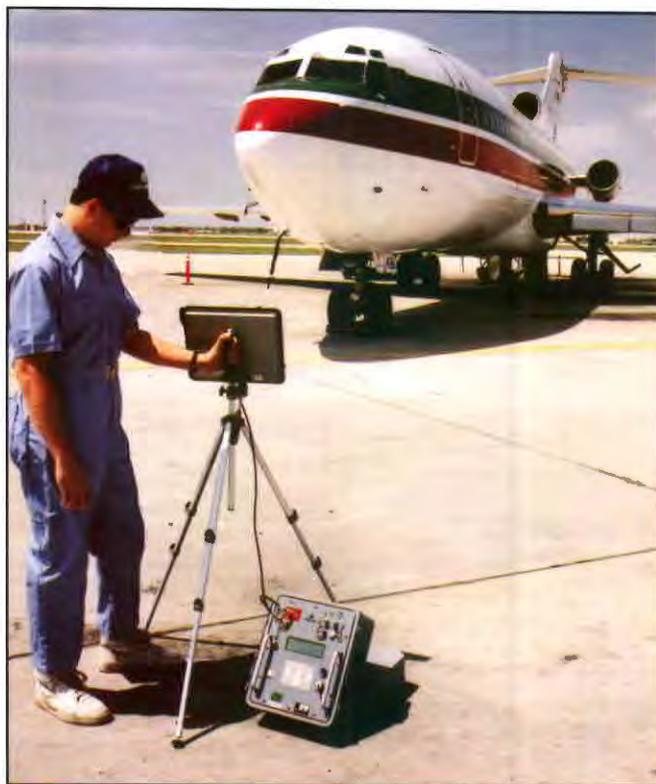
Tests to verify and certify a TCAS (Traffic Alert and Collision Avoidance System) can be done outside the airplane. The ramp tester, an Aeroflex TCAS-201, communicates with the airplane via radio signals and simulates different collision conditions. Without connecting directly into airplane systems it measures signal power, frequency, interrogations and replies. The tester is programmable to perform ten different collision scenarios.
