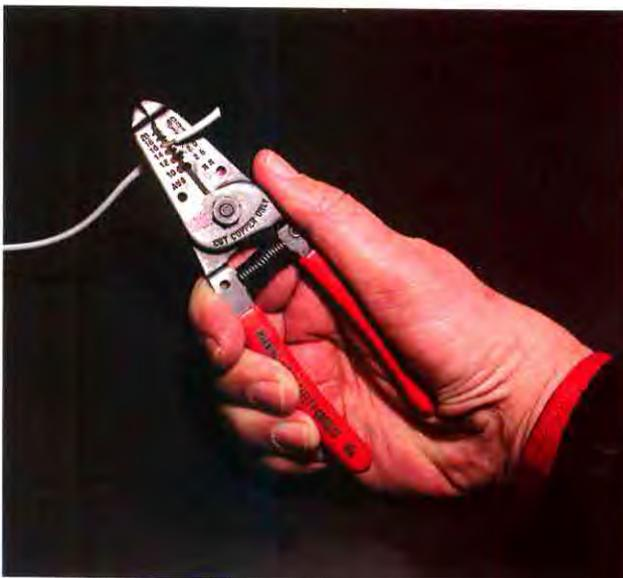
A wire stripper, like this manual type, should have notches to match different wire sizes. A high-quality stripper remains sharp and has a return spring. At the right is a semi-automatic stripper. It grips the wire as blades cut and remove the insulation.
