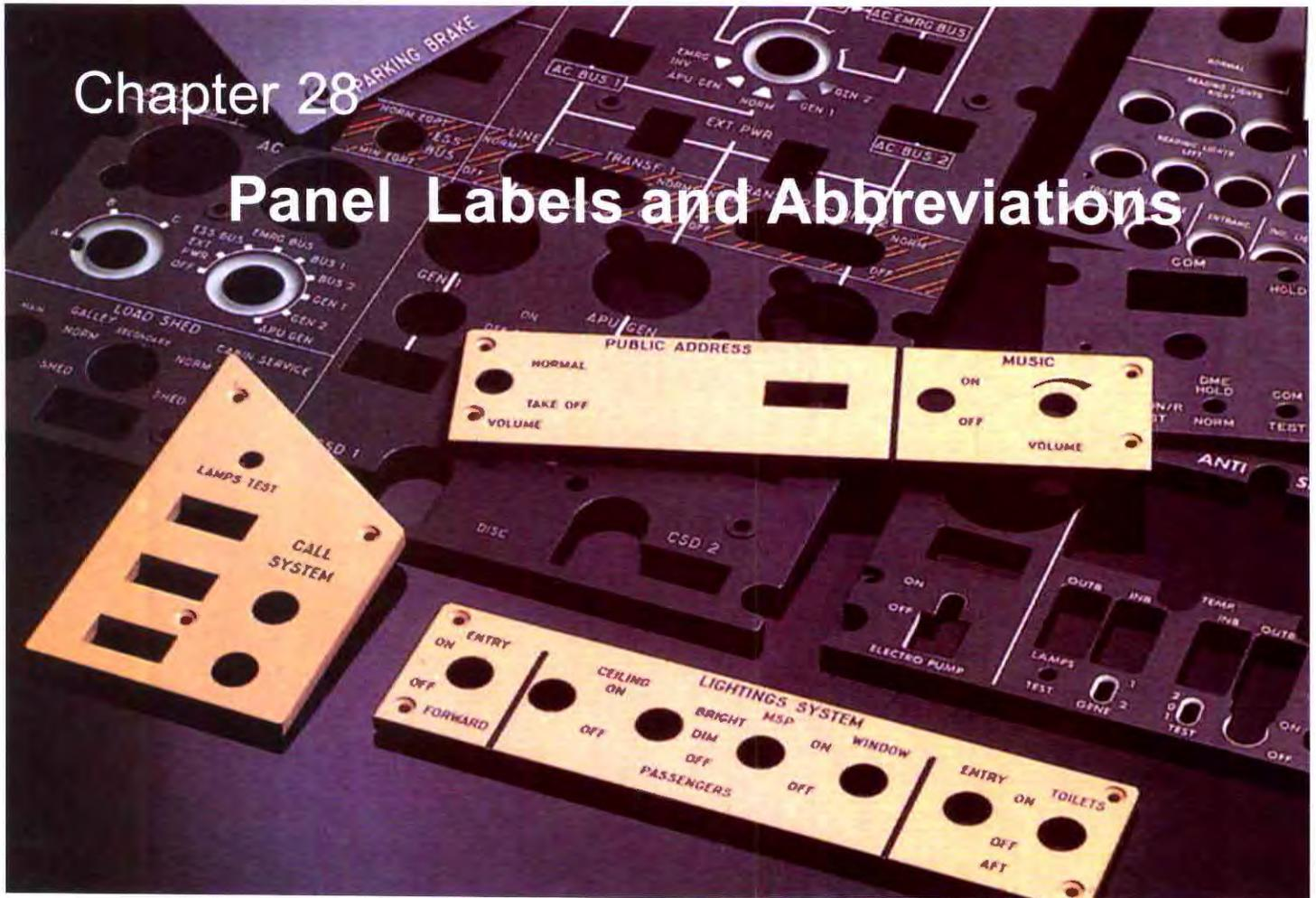
According to regulation, all controls and indicators on an airplane must be clearly labelled and visible to the pilot. Unmarked items can be handled several ways:
