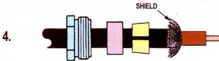
Push the shield back over the cable jacket.
