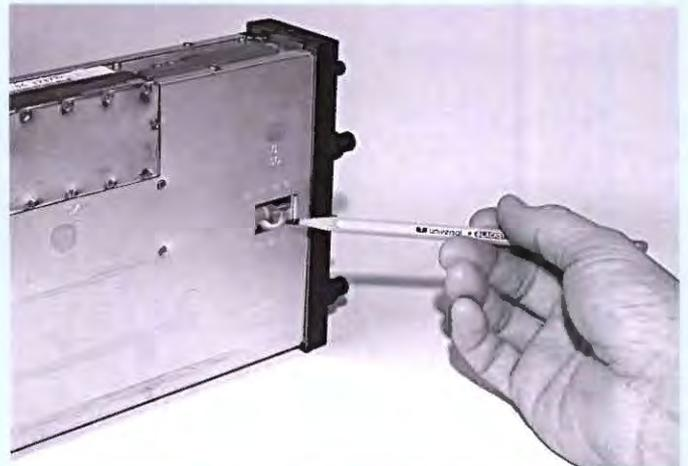
Pencil points to locking mechanism at underside of radio. As it turns, it engages a slot in the tray and pulls the radio in. To avoid damage, never force the radio into the tray.
