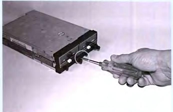
A panel-mounted radio is removed from the instrument panel by inserting a tool into an opening on the front. It may be a screwdriver, hex wrench or other tool.
