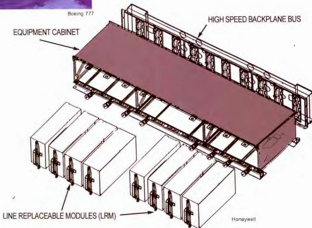
Integrated Modular Avionics (IMA) replace separate LRU's (line replaceable units), with LRM'S, "line replaceable modules." Unlike earlier systems, LRM's do not have one function per unit, such as receiver, transmitter, etc. They are more like computer resources that share and process information over a high speed databus. This provides smaller size and weight, and greater reliability.
