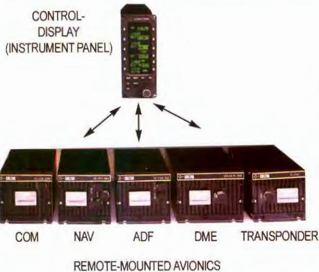
In remote-mounted avionics, only a control-display unit (CDU) is in the instrument panel; the rest is in a remote location. For small business aircraft, the location is often in the nose; larger jets have a compartment in the fuselage.
