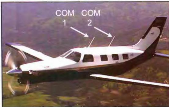
For most single-engine aircraft, com 1 and 2 antennas are located atop the cabin. Try to space them at least 36 inches apart to reduce interaction. This could reduce reception and transmission in certain directions.
