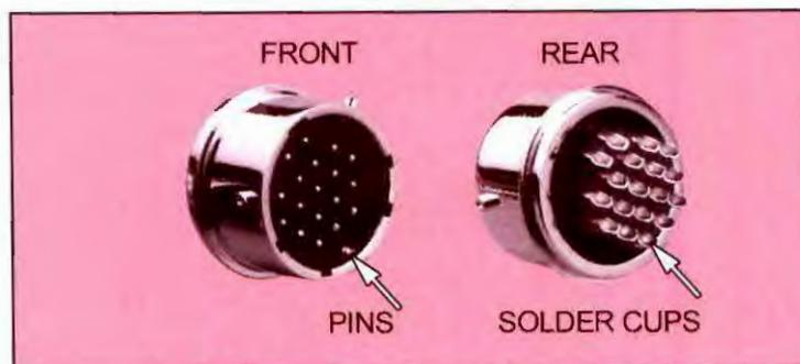
Wires to most connectors are crimped on, but some require soldering. The back of this connector has “solder cups” for holding solder and wire. After the connection is made, shrink-tubing is slid over bare wires to prevent short-circuiting.
